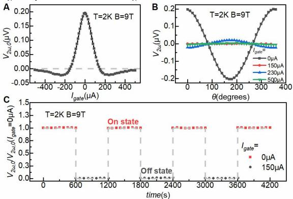
Fig. 3: Operation of a MnPS<sub>3</sub> magnon valve.
