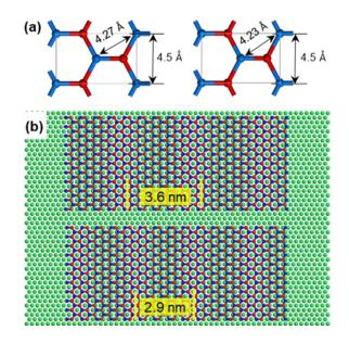
**Figure 4.** Structural models of CuSe on Cu(111) with different lattice distortions. (a) Unit cells of CuSe with lattice distortions. (b) CuSe on Cu(111) with 1D stripe structures by simply
