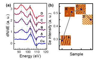
**Figure 5.** Auger electron spectroscopy of CuSe/Cu(111). (a) AES spectra of CuSe with different structures. The AES peaks for Cu and Se elements are denoted by solid and dashed lines, respectively. All the spectra are normalized by the peak-peak intensity of Cu at ~110 eV. The label A-D referred to samples A-D which are defined in Figs. 2 and 3. (b) AES intensity of Se for these samples.
