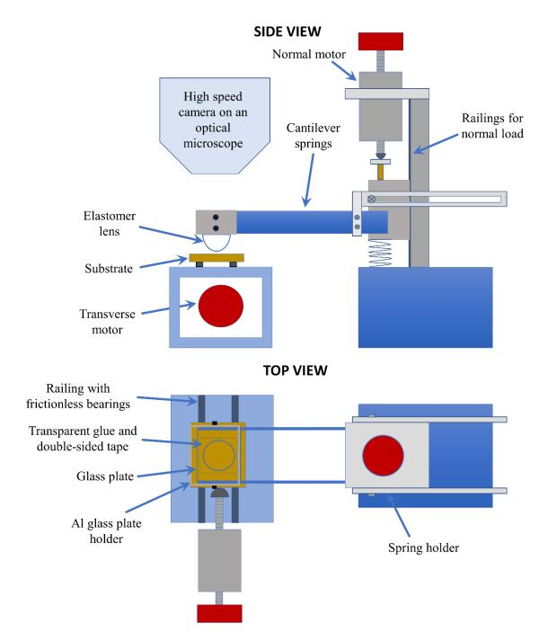
**Figure S3.** The double-cantilever setup for friction measurement through spring deflection and real-time area tracking through high-speed camera inspired by refs. [1,2].
