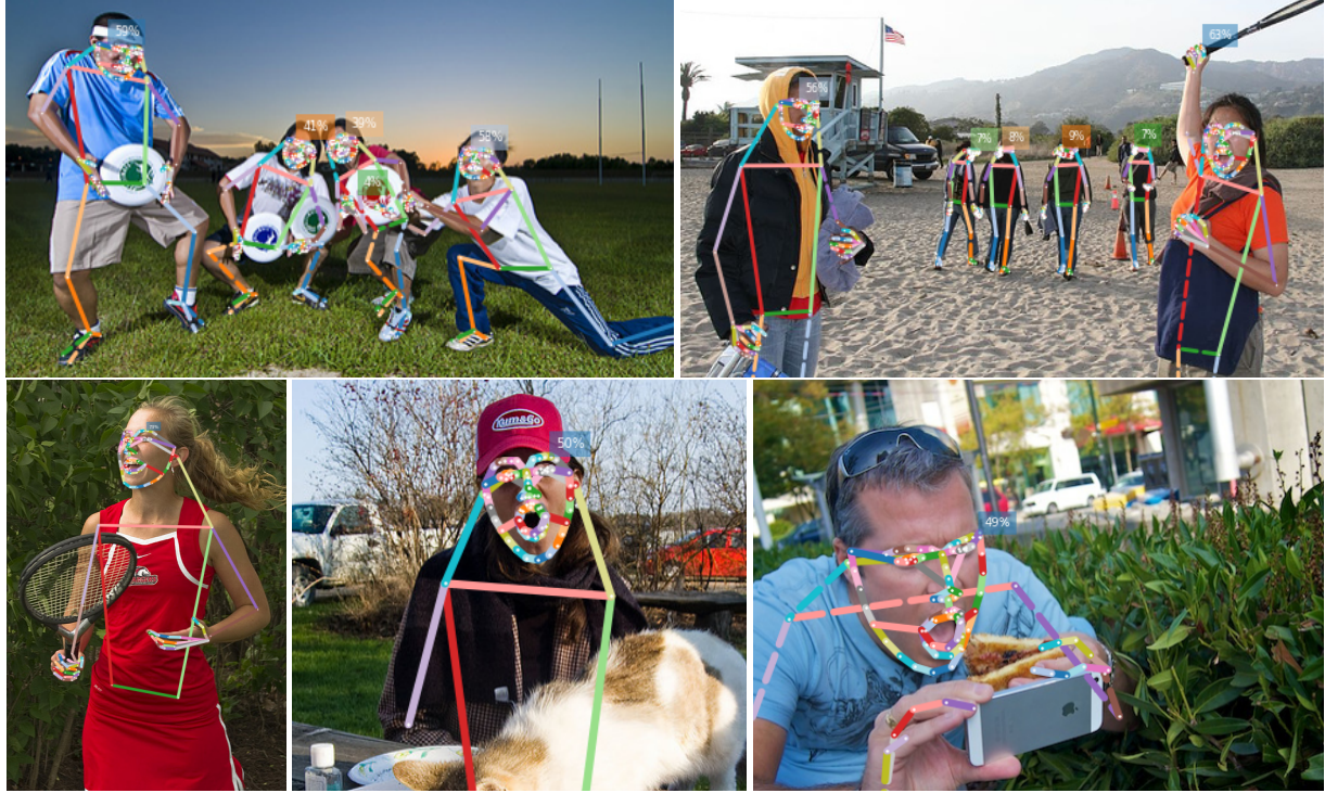
Figure 5: Qualitative results from the COCO WholeBody validation set [12]. Our method resolves multiple persons per image and captures their facial expressions and gestures like hailing a cab. The bottom-left image is processed with human and car pose estimators.
