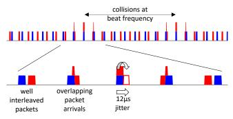
Fig. 5: periodic collisions between packet flows of different time domains; overlapping packet arrivals are served sequentially
