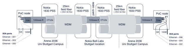
Fig. 19: Protocol stack, topology, and IXIA port mapping of the field trial experiment
