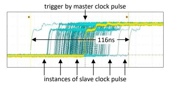
Fig. 17: Precision of PTP clock synchronization across a TDM reservation (oscillogram from [14]), recent results: mean master to slave pulse offset less than 1ns, standard deviation 5.9ns, peak-to-peak 64ns
