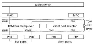
Fig. 9: Layer model of the combined TDM/packet node
