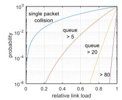
Fig. 3: Probability of waiting times. Large queues fade away at slightly reduced link load < 90%, while single packet collisions remain present even at low load.
