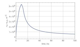
FIG. 7. A spatially averaged concentration of colloidal particles on the substrate surface as a function of time. Voltage  $\Phi = 0.5 V$ . The flows are switched on.
