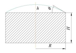
FIG. 1. Sessile droplet on a metal cylindrical substrate.
