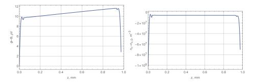
FIG. 6. Potential drop (on the left) and colloidal particle concentration curve as a function of z at r = 0.5R (on the right) at voltage 0.5 V. The flows are switched on.
