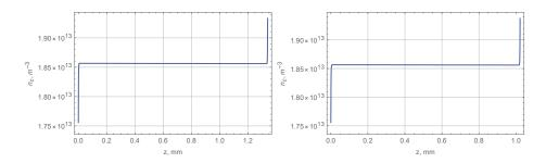
FIG. 5. Colloidal particle concentration curve as a function of z at r = 0 (on the left) and r = 0.5R (on the right) from the droplet center at the voltage  $\Phi = -0.5 V$ . The flows are switched off.
