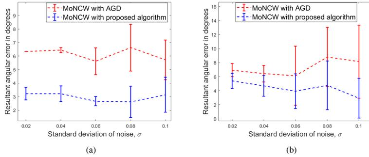
Figure 9: Mean and standard deviation of resultant angular error vs varying noise when fibers are oriented at (a)  $(\phi_1, \phi_2) = (10^\circ, 70^\circ)$  and (b)  $(\phi_1, \phi_2, \phi_3) = (0^\circ, 65^\circ, 130^\circ)$ . Polar angle is set to  $90^\circ$  for all fibers.
