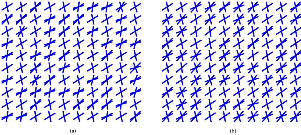
Figure 7: Estimation of fibers using (a) MoG with UGD and (b) MoG with proposed technique for 3-crossing fibers with  $(\phi_1, \phi_2, \phi_3) = (15^\circ, 55^\circ, 110^\circ)$  and noise,  $\sigma = 0.06$ . The weight fraction corresponding to each fiber is set to  $\frac{1}{3}$ .
