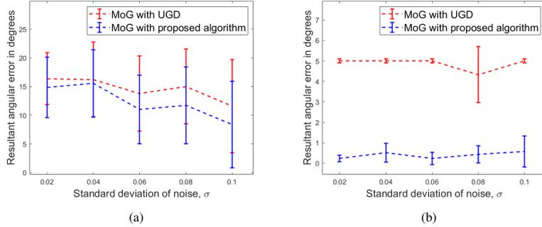
Figure 8: Mean and standard deviation of resultant angular error vs varying noise when fibers are oriented at (a)  $(\phi_1, \phi_2) = (10^\circ, 50^\circ)$  and (b)  $(\phi_1, \phi_2, \phi_3) = (50^\circ, 110^\circ, 170^\circ)$ . Polar angle is set to  $90^\circ$  for all fibers.
