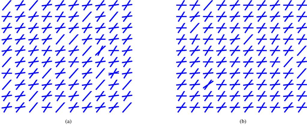
Figure 4: Estimation of fibers using (a) MoNCW with AGD and (b) MoNCW with proposed technique for 2-crossing fibers with  $(\phi_1, \phi_2) = (0^\circ, 60^\circ)$  and noise,  $\sigma = 0.06$ . The weight fraction corresponding to these fibers is set to 0.3 and 0.7 respectively.
