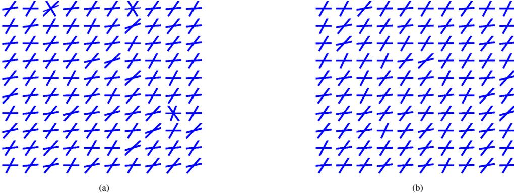
Figure 3: Estimation of fibers using (a) MoNCW with AGD and (b) MoNCW with proposed technique for 2-crossing fibers with  $(\phi_1, \phi_2) = (0^\circ, 60^\circ)$  and noise,  $\sigma = 0.1$ . The weight fraction corresponding to both the orientations is set to 0.5.
