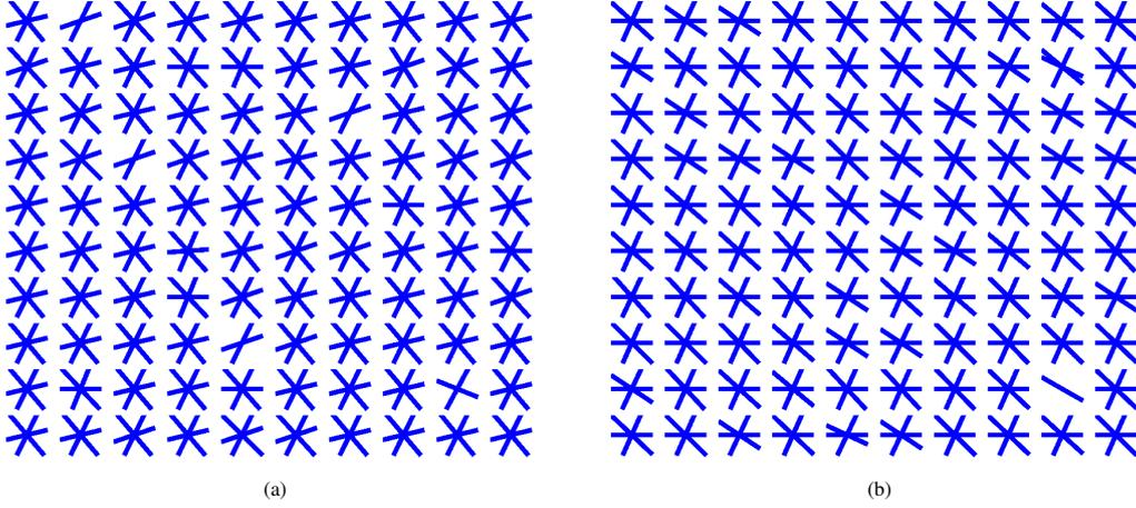
Figure 6: Estimation of fibers using (a) MoNCW with AGD and (b) MoNCW with proposed technique for 3-crossing fibers with  $(\phi_1, \phi_2, \phi_3) = (0^\circ, 65^\circ, 130^\circ)$  and noise,  $\sigma = 0.1$ . The weight fraction corresponding to each fiber is set to  $\frac{1}{3}$ .
