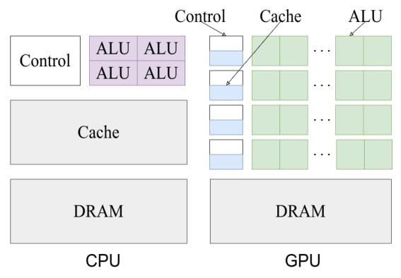
Figure 1.1: The structure of CPU and GPU [5].
