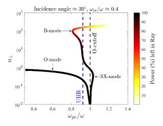
Figure 21, dispersion relation obtained from the ray-tracing calculation indicating the power absorption strength of the various wave branches. The microwave beam is injected with O-mode polarization. At that point, no absorption has occurred, and the power left on the beam is 100 %. The beam starts to lose power once it crosses the UHR layer as a SX-mode and the power left on the beam reaches 0% along the B-mode branch.
