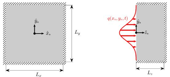
Figure 24, (left) front and (right) side view of the target plate geometry used to solve the heat diffusion problem. All surfaces have insulating boundary conditions except for the "front-side" surface which has an applied surface heat flux distribution  $q(x_*, y_*, t)$ .
