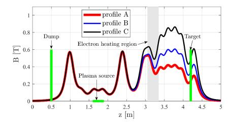
Figure 10, Magnetic field scenarios used to determine optimal magnetic field profile. Grey region illustrates the position of the 28 GHz microwave chamber (Figure 2).
