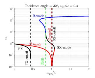
Figure 27, Same as Figure 26 (left) but with a ratio of  $\omega_{ce}/\omega = 0.4$ . Notice the different behavior of the B-mode.
