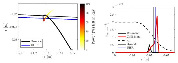
Figure 20, (left) close-up view illustrating the behavior of the ray near the Upper-Hybrid Resonance (UHR) layer and O-mode cutoff. (right) Radial profiles of plasma density and microwave absorption profiles in the electron heating chamber. Both resonant and non-resonant (collisional) absorption profiles are presented. The vertical lines represent the UHR and O-mode cutoff layers. Electron temperature is uniform with a value of 4 eV.
