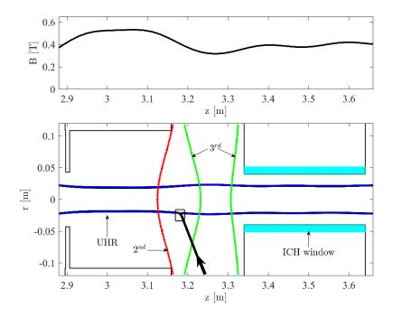
Figure 19, (top) On-axis magnetic field profile throughout the electron heating chamber. (bottom) schematic describing the ray-tracing calculation setup. Microwave beam is injected from the bottom at an incidence angle of 30 degrees. Red and green lines represent 2<sup>nd</sup> and 3<sup>rd</sup> harmonic resonance layers. The small rectangle encloses the region where strong absorption is observed (see Figure 20).
