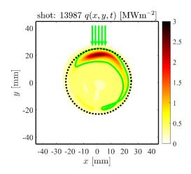
Figure 22, 2-D heat flux pattern at the target measured during 28 GHz electron heating experiments with oblique microwave injection. The green arrows indicate the location of the microwave injection. Experimental setup is described in reference [17]. The green contour line encloses about 1/3 of integrated heat flux.
