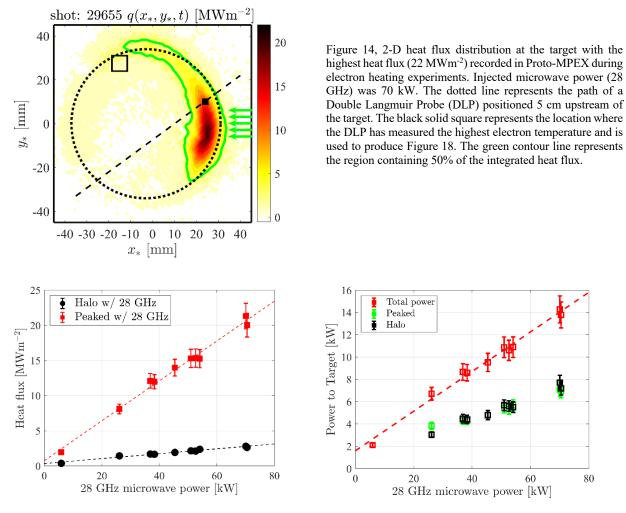
Figure 15, Heat flux (left) and total power (right) coupled to the target as a function of 28 GHz microwave power. The heat flux is measured in two different regions: (black circles) "halo" and (red squares) "peaked" region. The total power includes the contribution of both the 13.56 MHz and 28 GHz power. Lines represent best linear fits to the data.
