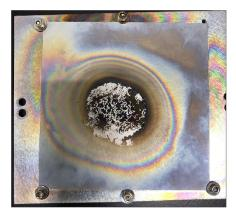
Figure 5, Example illustrating the surface modification and deposits formed on the "front-side" (plasma-exposed) surface of the tungsten target after multiple months of plasma operation. These features can introduce important changes to the surface IR emissivity and errors in the thermographic analysis. No IR emissivity changes were observed on the "back-side" surface of the target.
