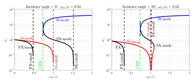
Figure 26, Cold-plasma wave dispersion for (left) perpendicular propagation (normal angle of incidence) and (right) oblique angle of incidence of 35 degrees. The blue line corresponds to the electron Bernstein wave (B-mode) and is calculated by solving the roots of Eq. 26. A ratio of  $\omega_{ce}/\omega = 0.52$  is used.
