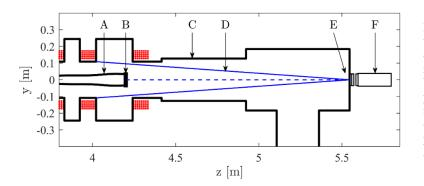
Figure 4, 1:1 scale schematic of the target plate and IR thermographic diagnostic setup. Labelled items represent the following: (A) plasma boundary (LUFS), (B) tungsten target plate, (C) vacuum boundary, (D) light rays representing the Field Of View (FOV) of the IR camera, (E) viewing port with ZnSe window and (F) FLIR A655 IR camera.
