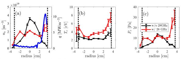
Figure 17, Radial (a) electron density, (b) electron temperature and (c) electron pressure profiles measured with a Double Langmuir Probe (DLP) 5 cm upstream of the tungsten target along the path shown in Figure 14. The dotted vertical lines represent the LUFS. The blue trace in (a) represents the IR-based heat flux on the target along the path shown in Figure 14.
