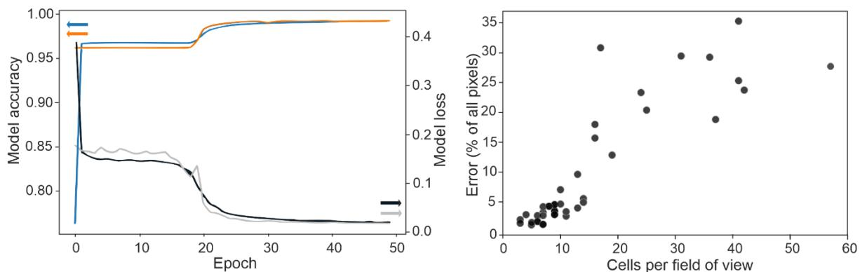
**Figure S5:** A) The accuracy and loss of the segmentation model plotted against iterative epoch for the training images (blue, black respectively) and validation images (orange, grey respectively) using the U-Net with optimal parameters; B) rate of classification error for pixels in image against number of cells per field of view for all experimental datasets.
