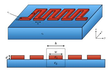
FIG. 6. Top: schematic of an superconducting nanowire single-photon detector (SNSPD) consisting of a superconducting wire meander (red) deposited on an electrically insulating substrate (blue). Bottom: two-dimensional cross section (fixed z) of the SNSPD.
