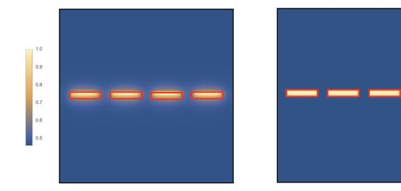
FIG. 7. Numerical solution for the response function  $\psi(x, y)$ , discussed in Sec. V B for a periodic array of rectangular crosssection wires (depicted by red rectangles) and  $k_z d = 1$  (*left panel*),  $k_z d = 10$  (*right panel*), where d is the wire thickness. Orange corresponds to higher magnitudes for  $\psi$ , and blue to smaller magnitudes (color bars are in arbitrary units).
