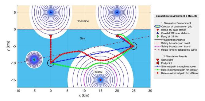
Figure 3. Comparison of path planning for NIB-enabled ship fleet in maritime network. NIB-embodied ship fleet travel from start point to end point through two waypoints at maximum speed of 30 km/h. The ferry with shipborne WiFi passes on the route across the simulation region at the constant speed of 40 km/h.
