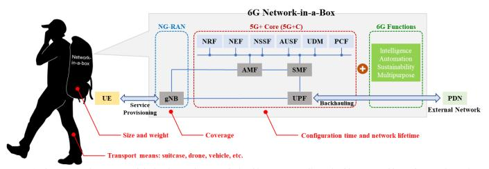
Figure 1. The conceptual structure and the key factor of an easy-deployable NIB potentially applicable to 5G and beyond (5G+) that make an NIB different from traditional wireless network. The acronyms of network functions in 5G can be found in [9], while UE, gNB and PDN stand for user equipment, new generation Node B, and packet data network. This structure also works for future 6G.
