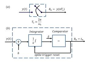
Fig. 1. (a) classical schematic sampler. (b) IF-TEM sampler.
