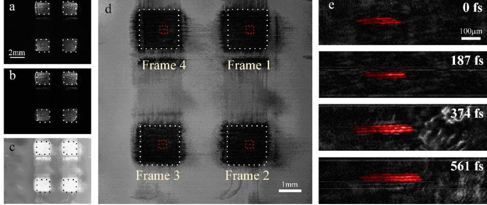
Fig.5 a) four frames with dynamic of laser-induced plasma; b) four frames without dynamic events; c) the image processed based on equ.3; d) the image with further processing; e) dynamic of laser-induced plasma with framing time 187fs.
