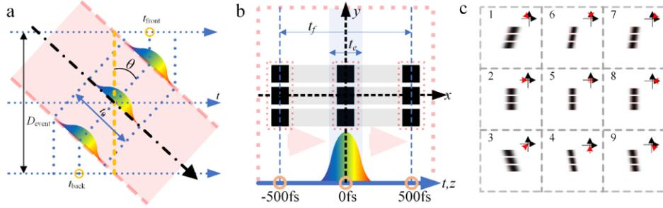
Fig.6 a) Illumination schematic diagram; b) dynamic event schematic diagram. c) the results of the nine frames simulation with different directions of incidence projecting on x-y plane, along: 1)  $-45^\circ$ ; 2) x-axis; 3)  $45^\circ$ ; 4) y-axis; 5) z-axis; 6) minus y-axis; 7)  $-135^\circ$ ; 8) minus x-axis; 9)  $135^\circ$ .
