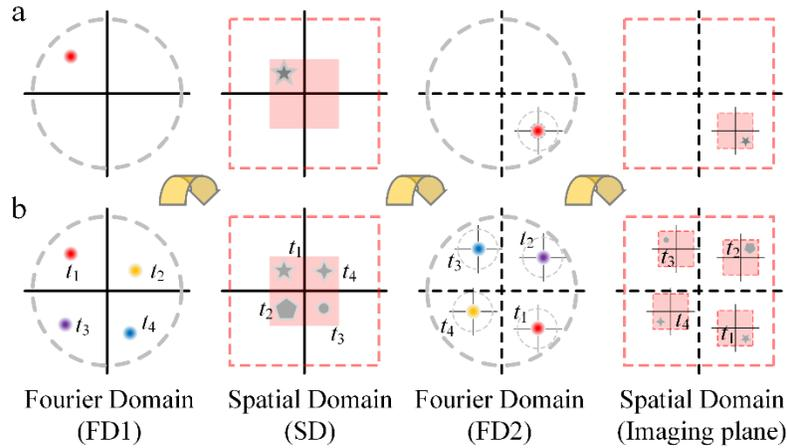
Fig.1 The operating principle of the FIP system: a) the principle of I4F; b) the principle of FIP.
