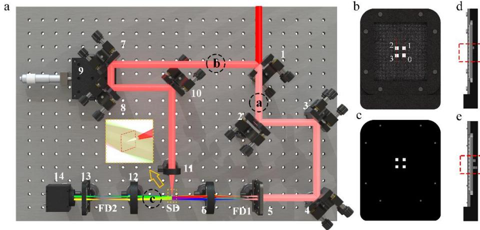
Fig.4 a) Schematic diagram of experimental set-up: (1). beam splitter mirror; elements (2), (3), (4), (7), (8), (10) are mirrors; (5). Integrated framing structure: LA1 and step array; (6). L1; (9). translation stage; (11). convergent lens; (12). L2; (13). LA2; (14). detector. b) left view of the integrated framing structure; c) right view of the integrated framing structure; d) section view at steps 1 and 2; e) section view at steps 3 and 4.
