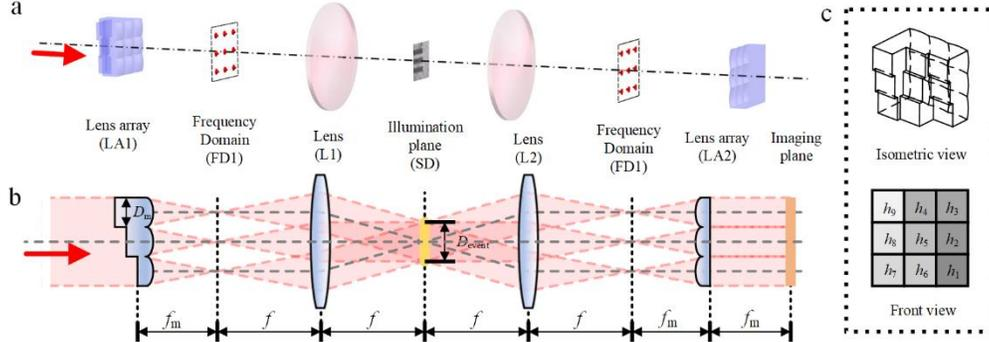
Fig.2 a) The 3D model of FIP system; b) light path diagram of FIP system; c) isometric and front view of framing structure.
