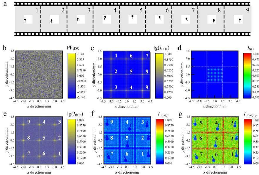
Fig.3 The system was simulated in a single shot, a) the intensity distribution in FD1; b) the intensity distribution in SD; c) the intensity distribution in FD2; d) the phase distribution in FD2; e) the intensity distribution in imaging plane; f) the related intensity distribution after processing; g) 9 frames of the simulated dynamic event.
