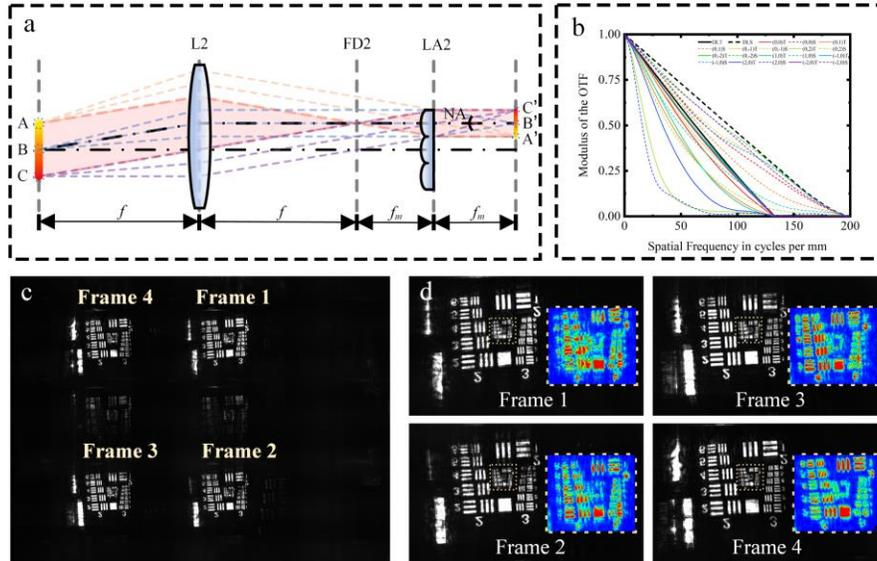
Fig.8 a) Imaging structure schematic diagram; b) MTF of the experiment system; c) the measured image; d) details for four frames (Colorful maps in each frame show the group 4 and 5 of the USAF 1951 optical resolution).
