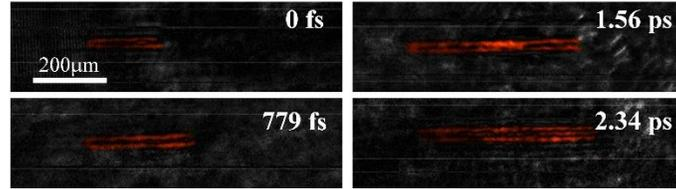
Fig.7 Dynamic of laser-induced plasma with 779 fs framing time
