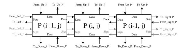
Fig. 4. Horizontal configuration of three adjacent cells. The dark gray and light gray lines show data and sign interconnections respectively.
