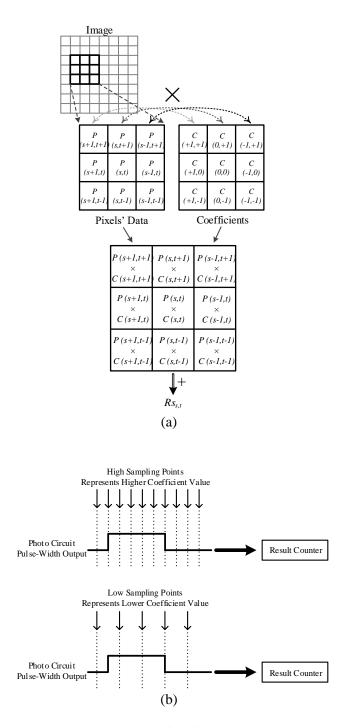
Fig. 1. a) Kernel convolution concept for a typical  $3 \times 3$  kernel size, b) A simple view of the sampling procedure.
