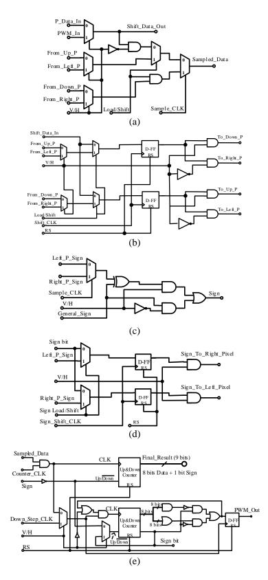
Fig. 2. Proposed processor circuit. a) Sampler, b) Data-Shifter, c) Sign-Generator, d) Sign-Shifter, and e) Result Counter
