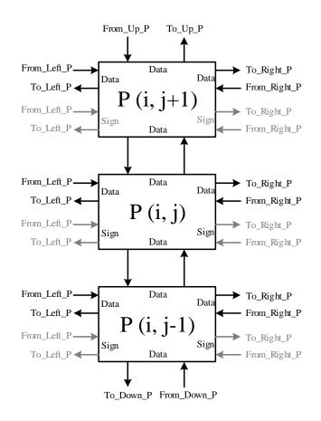
Fig. 3. Vertical configuration of three adjacent cells. The dark gray and light gray lines show data and sign interconnections respectively.
