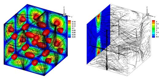
Figure 1: Isosurfaces of vorticity amplitudes and velocity streamtraces of LSF given by Eqs. (4) as the initial field (left) and decaying to a state with developed multi-scale excitations (right).
