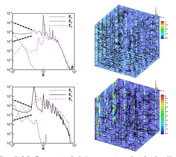
Figure 2: Left: Power spectra of velocity components, accelerated at  $k \approx 10$  (Ma = 0.1: upper row) and  $k \approx 5$  (Ma = 1: lower row), with the thick dashdot lines of, respectively,  $k^{-5/3}$  (K67) and k (equipartition in 2-space) spectra indicating that  $E_2$  appear in between; right: Isosurfaces of vorticity amplitudes and velocity streamtraces corresponding to the left-panel spectra.
