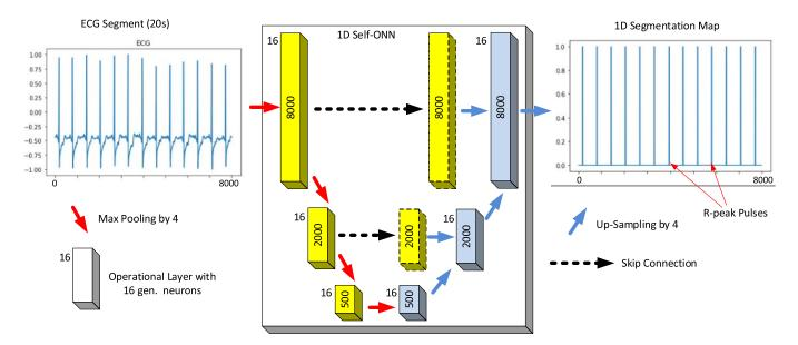
Fig. 4. Proposed approach for R-peak detection.
