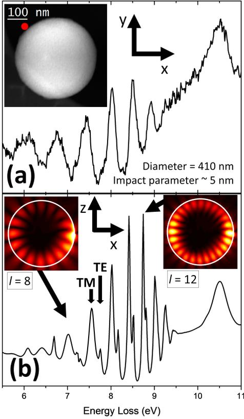
FIG. 1. (a) Experimental and (b) Simulated electron energy-loss spectra for an electron probe located  $\sim 5$  nm beside a 410 nm silica sphere. Inset in (a) displays a STEM image of the silica nanoparticle with the location of the electron probe (red dot). Insets in (b) display  $|H|$  maps for  $l = 8$  and  $l = 12$  on the  $x$ - $z$  plane (see text) with an electron travelling on the right of the sphere.
