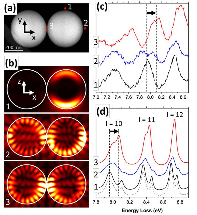
FIG. 2. (a) STEM image of silica bisphere with electron probe locations for  $|H|$  maps displayed in (b), experimental spectra displayed in (c) and simulated spectra displayed in (d). A simulated spectrum for an individual sphere is shown as a dotted line in (d).  $|H|$  maps are displayed on the  $x$ - $z$  plane that includes both center of the spheres. Locations 1 and 2 are  $\sim 5$  nm from the sphere's surface
