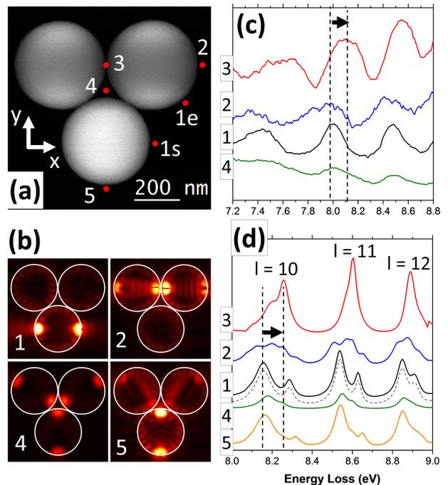
FIG. 3. (a) STEM image of a silica-sphere trimer with electron probe locations for  $|H|$  maps displayed in (b), experimental spectra displayed in (c) and simulated spectra displayed in (d). A simulated spectrum for an individual sphere is shown as a dotted line in (d).  $|H|$  maps are displayed on the  $x$ - $y$  plane that includes the centers of the spheres. Locations 1, 2 and 5 are  $\sim 5\text{nm}$  from the sphere's surface
