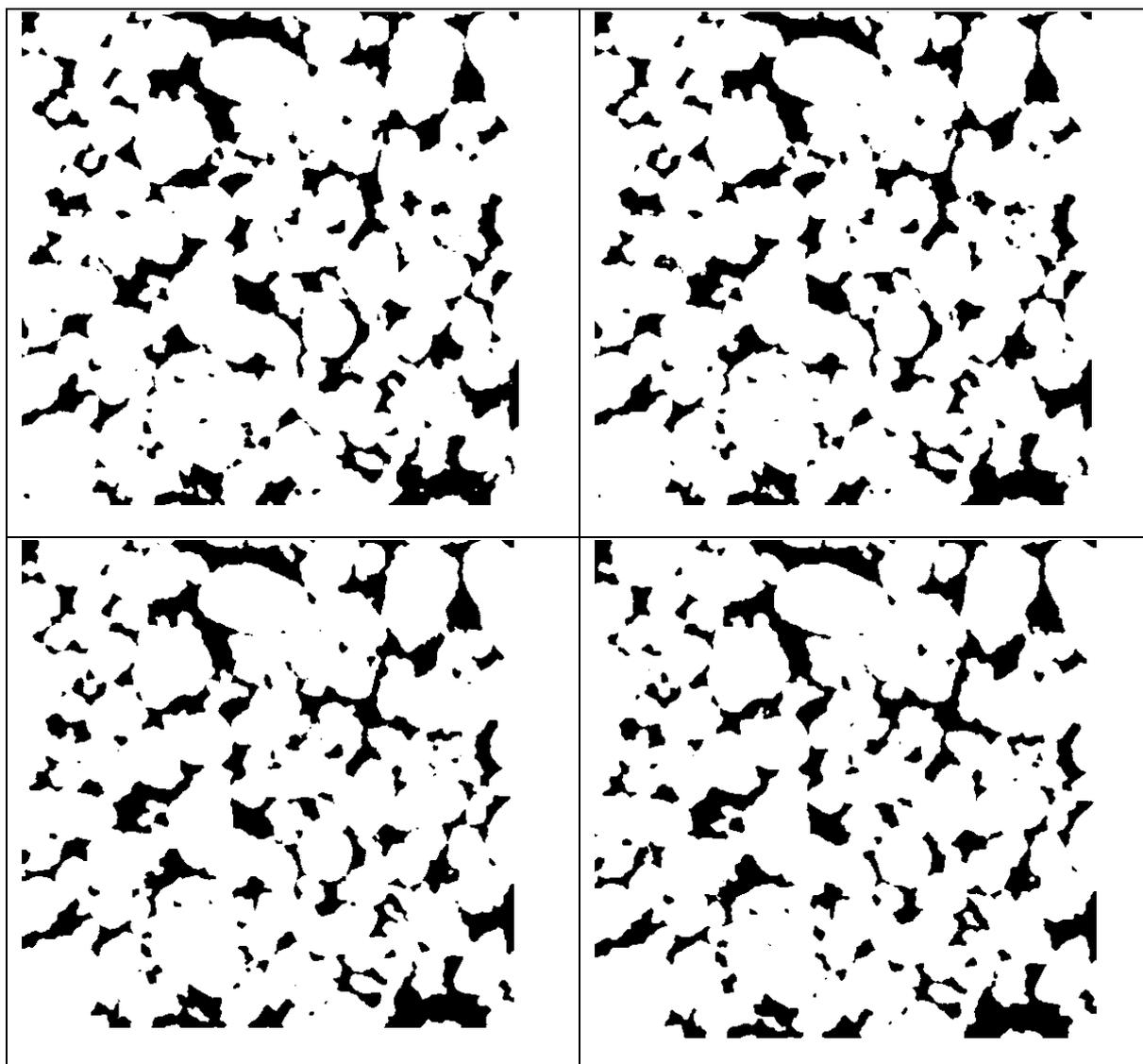
**Figure 1:** Cross sections of the 3D binary image representing pore space (pore space voxels are colored black) ; the order is left to right and up to bottom
