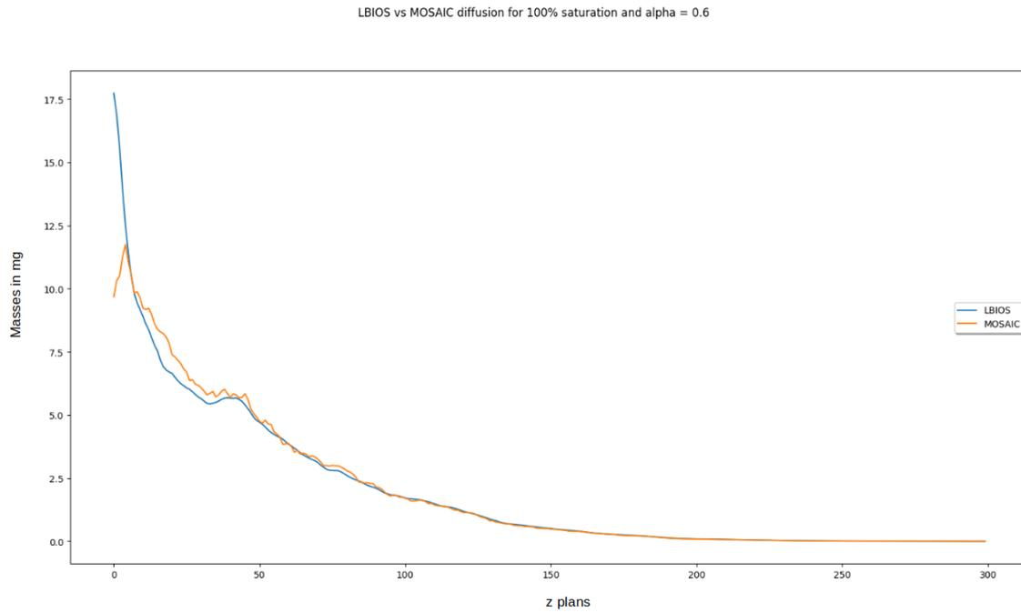
**Figure 7:** Comparison of the diffusion simulation results MOSAIC/LBIOS ; MOSAIC curve is blue colored ; LBIOS curve is red colored ; the area of the contact surface for MOSAIC diffusion is set to  $0.6 \cdot s_{\min}(i,j)$  ; the normalized intercorrelation between the two curves is around 0.98 ; the water saturation is 100% ; X-axis: number of the plane (0 to 299) ; Y-axis: total mass of DOM within the plane (expressed in mg).
