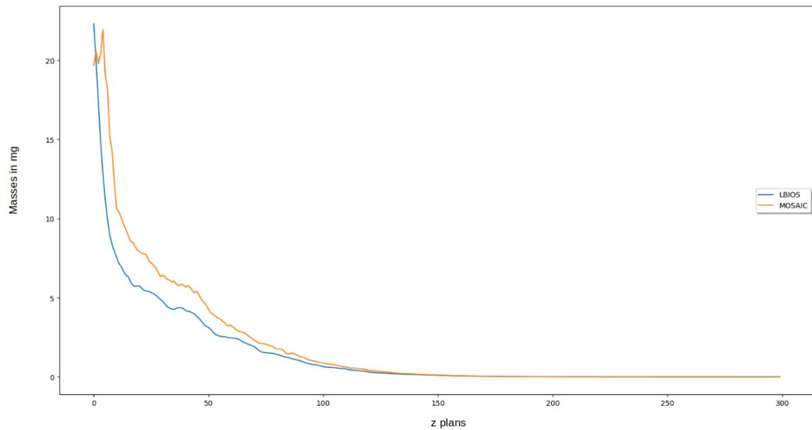
**Figure 9:** Comparison of the diffusion simulation results MOSAIC/LBIOS ; MOSAIC curve is blue colored ; LBIOS curve is red colored ; the area of the contact surface for MOSAIC diffusion is set to  $0.6 \cdot s_{\min}(i,j)$  ; the normalized intercorrelation between the two curves is around 0.98 ; the water saturation is 50% ; X-axis: number of the plane (0 to 299) ; Y-axis: total mass of DOM within the plane (expressed in mg).
