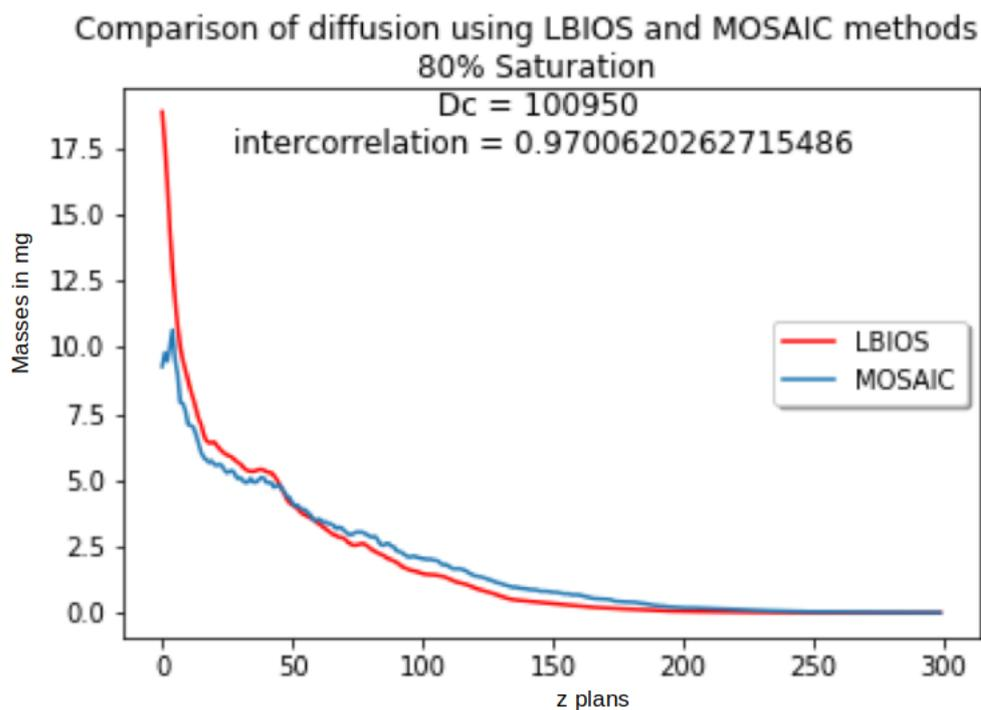
**Figure 12:** Comparison of the diffusion simulation results MOSAIC/LBIOS ; MOSAIC curve is blue colored ; LBIOS curve is red colored ; the area of the contact surface for MOSAIC diffusion is set to  $\text{smin}(i,j)$  ; the normalized intercorrelation between the two curves is around 0.97 ; the water saturation is 80% ; X-axis: number of the plane (0 to 299) ; Y-axis: total mass of DOM within the plane (expressed in mg).
