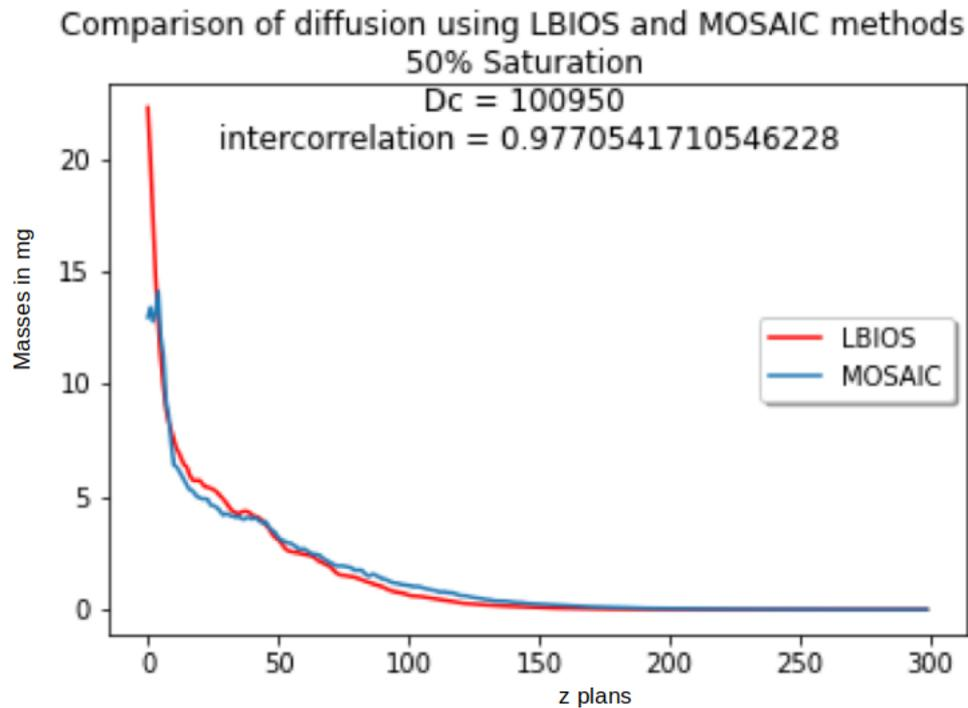
**Figure 13:** Comparison of the diffusion simulation results MOSAIC/LBIOS ; MOSAIC curve is blue colored ; LBIOS curve is red colored ; the area of the contact surface for MOSAIC diffusion is set to  $\text{smmin}(i,j)$  ; the normalized intercorrelation between the two curves is around 0.98 ; the water saturation is 50% ; X-axis: number of the plane (0 to 299) ; Y-axis: total mass of DOM within the plane (expressed in mg).
