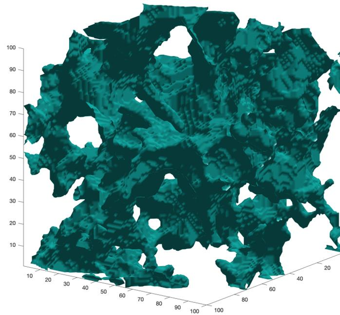
**Figure 2:** Perspective view of 3D pore space using Matlab routine (pore space is colored green)
