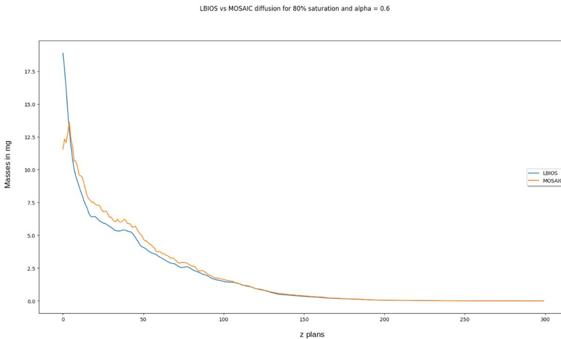
**Figure 8:** Comparison of the diffusion simulation results MOSAIC/LBIOS ; MOSAIC curve is blue colored ; LBIOS curve is red colored ; the area of the contact surface for MOSAIC diffusion is set to  $0.6 \cdot \text{sm}(\mathbf{i}, \mathbf{j})$  ; the normalized intercorrelation between the two curves is around 0.98 ; the water saturation is 80% ; X-axis: number of the plane (0 to 299) ; Y-axis: total mass of DOM within the plane (expressed in mg).
