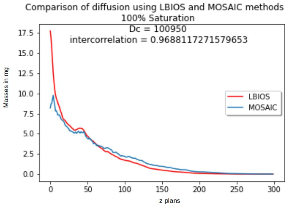
**Figure 11:** Comparison of the diffusion simulation results MOSAIC/LBIOS ; MOSAIC curve is blue colored ; LBIOS curve is red colored ; the area of the contact surface for MOSAIC diffusion is set to  $\mathbf{smin(i,j)}$  ; the normalized intercorrelation between the two curves is around 0.97 ; the water saturation is 100% ; X-axis: number of the plane (0 to 299) ; Y-axis: total mass of DOM within the plane (expressed in mg).
