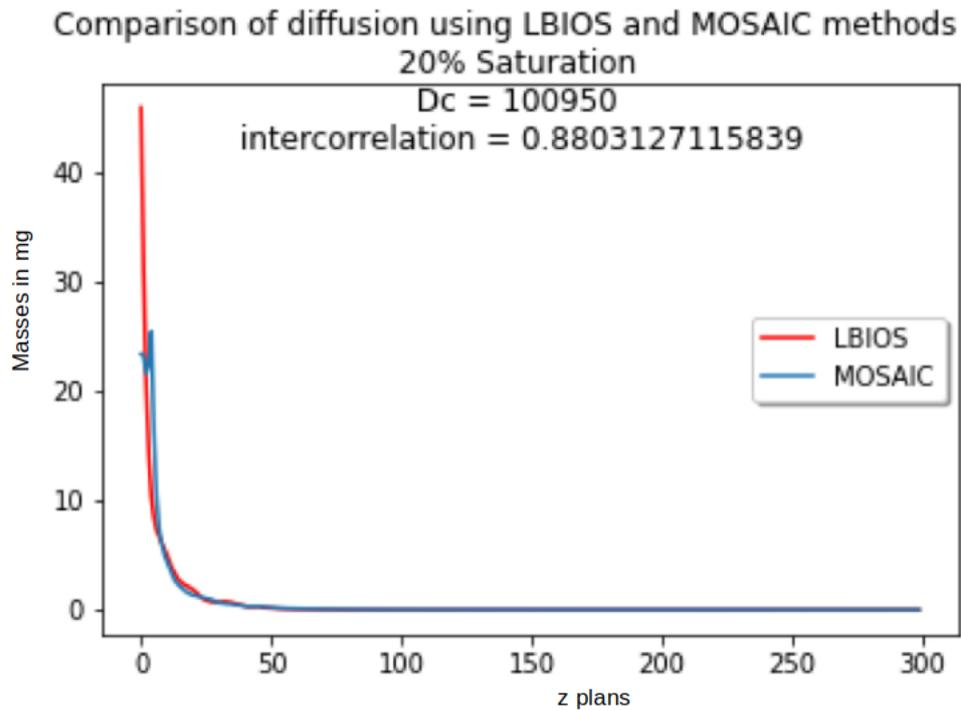
**Figure 14:** Comparison of the diffusion simulation results MOSAIC/LBIOS ; MOSAIC curve is blue colored ; LBIOS curve is red colored ; the area of the contact surface for MOSAIC diffusion is set to  $\mathbf{smin(i,j)}$  ; the normalized intercorrelation between the two curves is around 0.88 ; the water saturation is 20% ; X-axis: number of the plane (0 to 299) ; Y-axis: total mass of DOM within the plane (expressed in mg).
