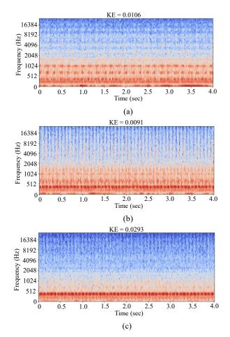
**Fig. 2.** Log Mel-spectrogram of original acoustic signals: (a) normal, (b) outer race fault 1.0 mm, and (c) inner race fault 1.0 mm.
