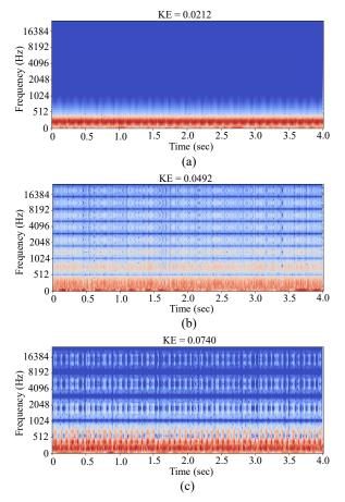
Fig. 3. Log Mel-spectrogram of denoised acoustic signals: (a) normal, (b) outer race fault 1.0 mm, and (c) inner race fault 1.0 mm.
