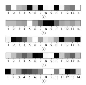
**Fig. 4.** Normalized statistical-spectral acoustic features after adaptive wavelet denoising: (a) normal, (b) outer race fault 0.3 mm, (c) outer race fault 1.0 mm, (d) inner race fault 0.3 mm, and (e) inner race fault 1.0 mm.
