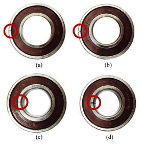
**Fig. 1.** Fault seeding of ball bearing: (a) outer race fault 0.3 mm, (b) outer race fault 1.0 mm, (c) inner race fault 0.3 mm, and (d) inner race fault 1.0 mm.
