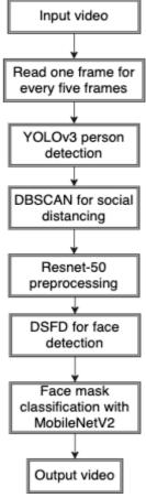
Fig. 4. System flow diagram
