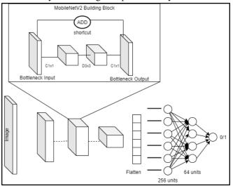
Fig. 10. MobileNetV2 model architecture
