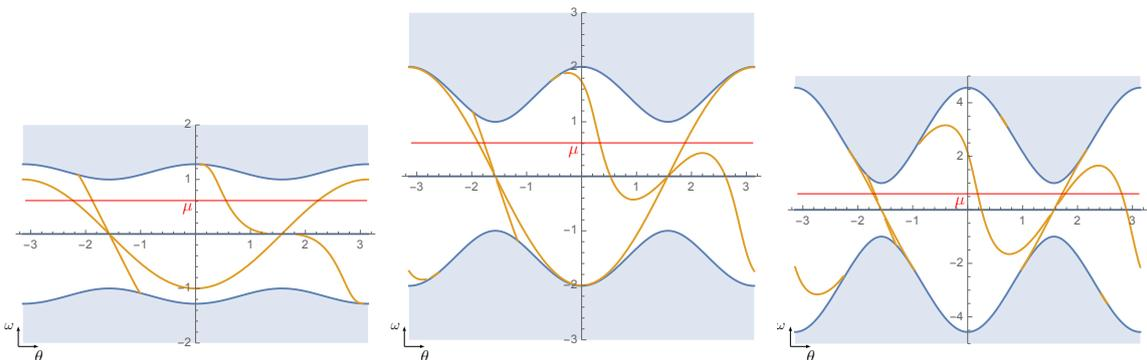
Figure 3: Spectrum of  $H_{R,\theta}^\sharp$  for  $f = 1$  and  $\epsilon = 0.2$ , along  $\mathcal{C}_R$  with  $R = 1, 2$  and  $4$ , respectively on the left, middle and right. Shaded blue regions correspond to extended solutions whereas yellow branches are edge modes confined near the boundary. The number  $n(\mathcal{C}_R, \mu)$  of signed intersections of such branches with the red line  $\omega = \mu$  is always 2, for any choice of  $R > 0$  and  $\mu \in (0, f)$ .
