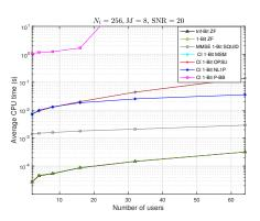
Fig. 4. CPU time versus the number of users, where  $N_t = 256$ , M = 8, and SNR= 20.
