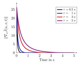
Fig. 4. Convergence of  $\nabla_u \tilde{J}(u, x, t)$  for different settling-times.
