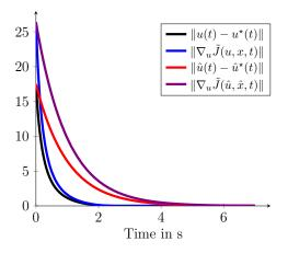
Fig. 1. Exponential and fixed-time convergence of tracking error and gradient of objective function.
