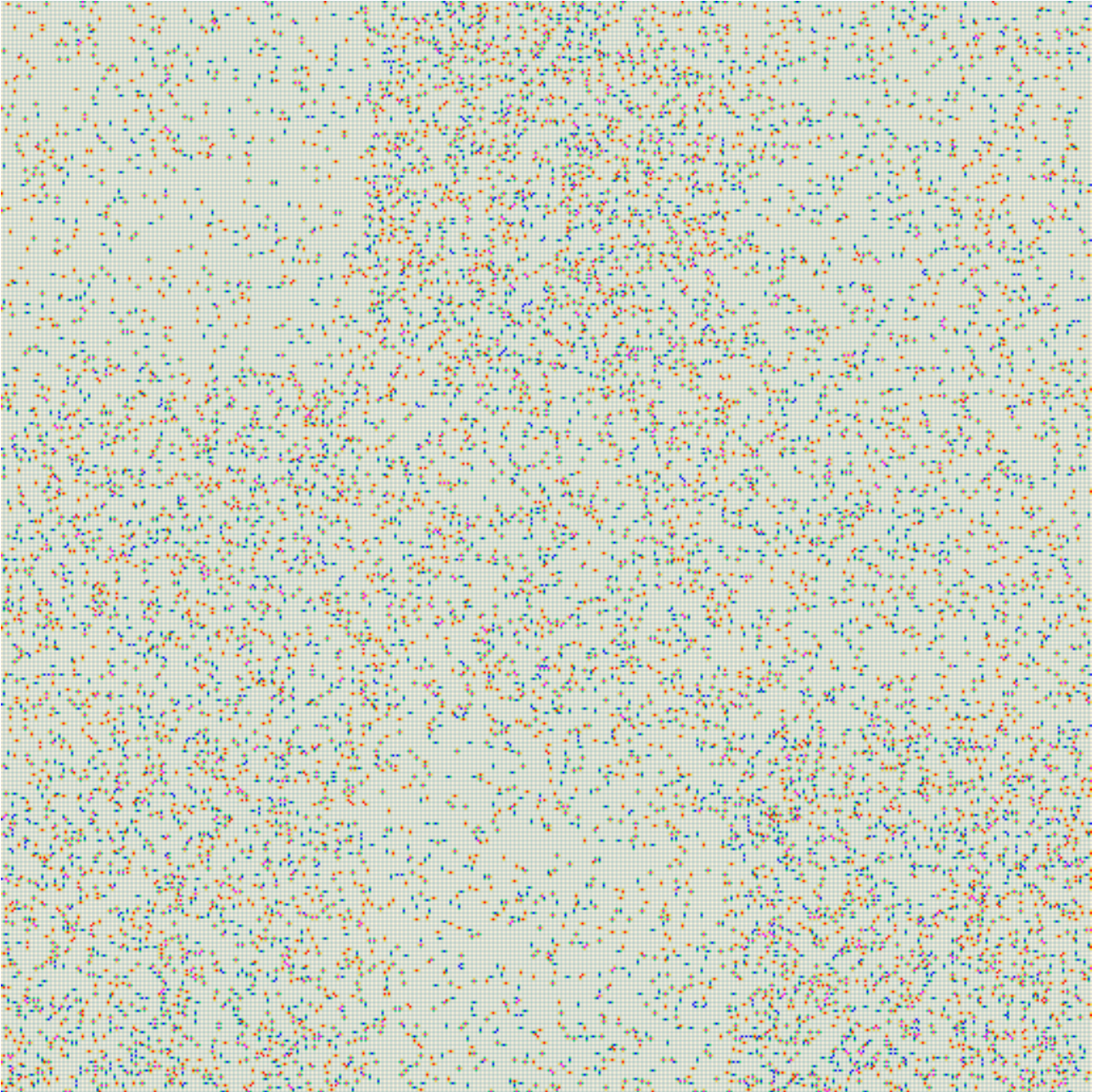
Figure 25: An example of distance 257 surface code subject to spatially inhomogeneous noise where the board is divided into nine patches with depolarising noise levels of 4%, 11%, 6%, 9%, 8%, 7%, 1%, 5% and 12%.
