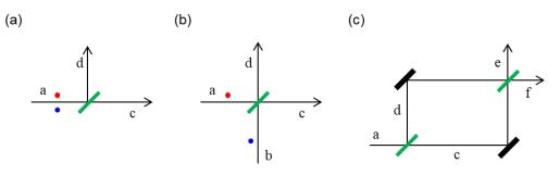
Fig. 1. Schematics of BS interacting with single photons. (a) For the same input port. (b) For the different input ports. (c) Mach-Zehnder interferometer with the same input. The red and blue dots indicate input photons.
