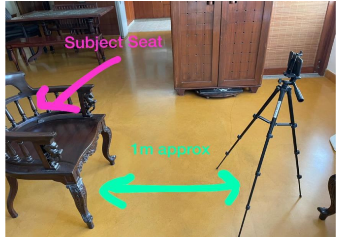
Fig. 14: Depiction of set-up for video data acquisition.
