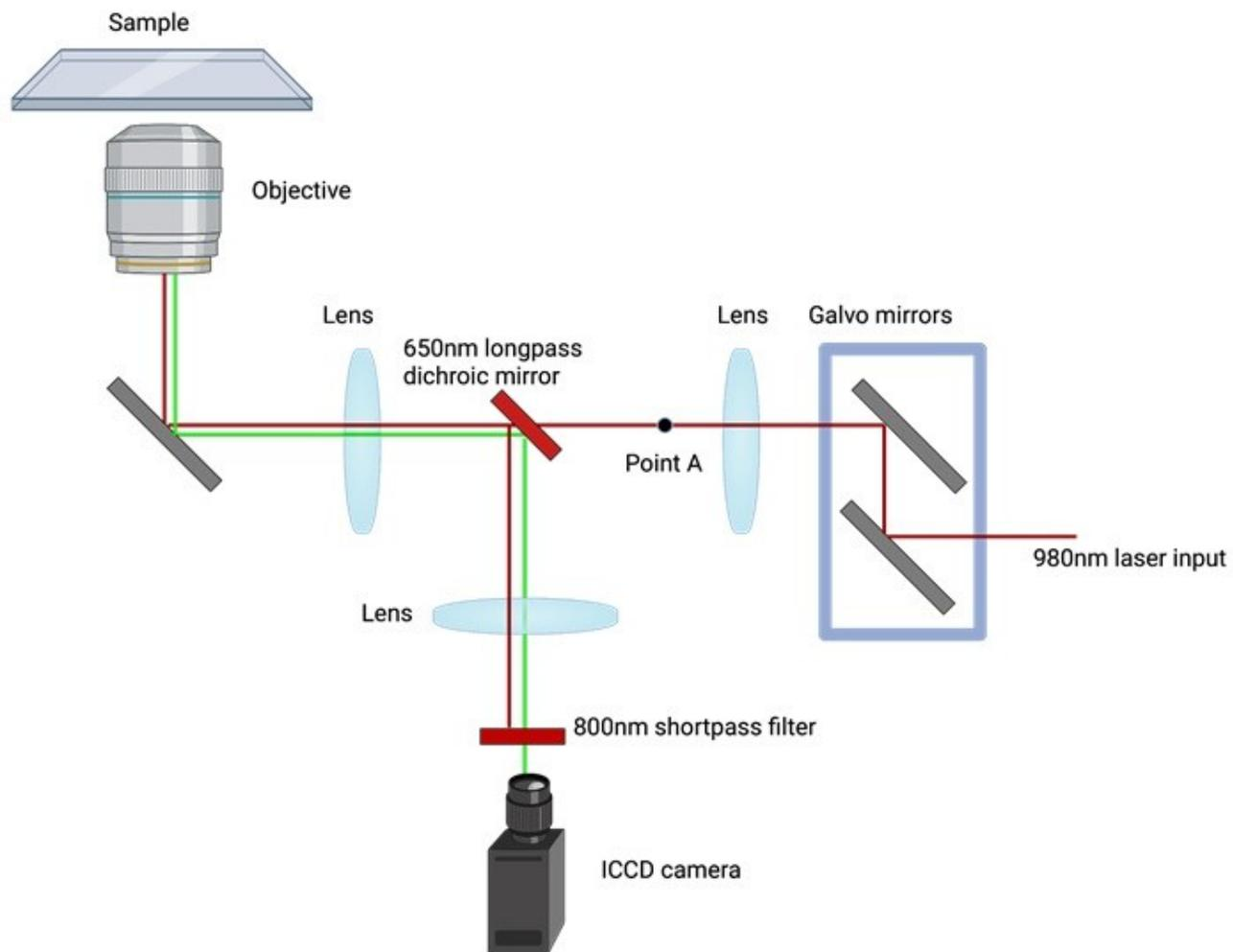
**Figure S2** – Wide field fluorescence imaging setup schematic. Using galvo mirrors, the laser is moved on the sample in a raster scan. The ICCD camera collects the signal from each point of the raster scan during the whole time of the scan.
