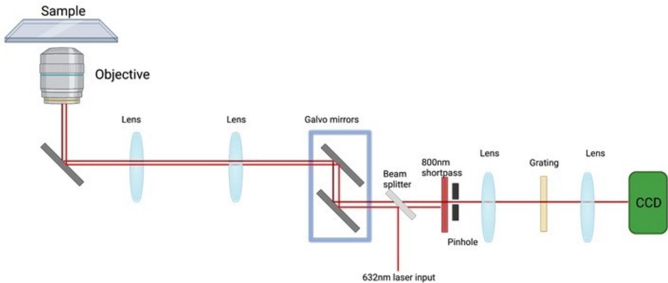
**Figure S1** – Confocal spectroscopy and microscopy setup schematic. Using the galvo mirrors, the 632 nm laser is moved on the sample in a raster scan. A 632 nm notch filter (shown in red rectangle before pinhole) blocks the laser residual reflection. The image of the pinhole is blown through a transmission grating 300 lines/mm and imaged on an ICCD camera. The pixel counts are then transformed to spectrum data.
