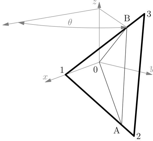
Figure 1: Calculation of integration limits as intersections of plane through origin with face 123 of tetrahedron
