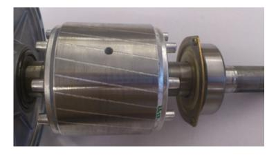
Figure 8. Induced rotor and bearing fault.
