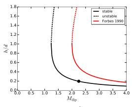
**Figure 3.** The locations of equilibria for the ratio  $\frac{h}{d}$  as a function of the relative strength of the dipole  $M_{\rm dip}$ . Black-solid portion of the line represents stable equilibria, while black-dashed portion unstable ones. Red lines display the same example but neglecting the gravity. The equilibria indicated by the black lines and the stable point chosen at  $M_{\rm dip} = 2.25$  correspond specifically to Case 3 defined in Section 2.1.2.
