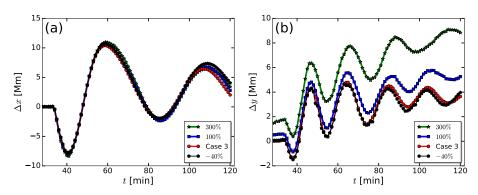
Figure 8. Test to determine weather the damped motion exhibited by the filament is due to numerical diffusion or it has a physical origin. Four runs were performed varying the spatial resolution, corresponding to relative coarser grids of 300%, 100% with respect to the standard resolution of Case 3, and a relative finer grid of -40%. We concluded that the acting damping process has a significant physical meaning. (a)–(b) Show horizontal and vertical displacements for the different resolutions.
