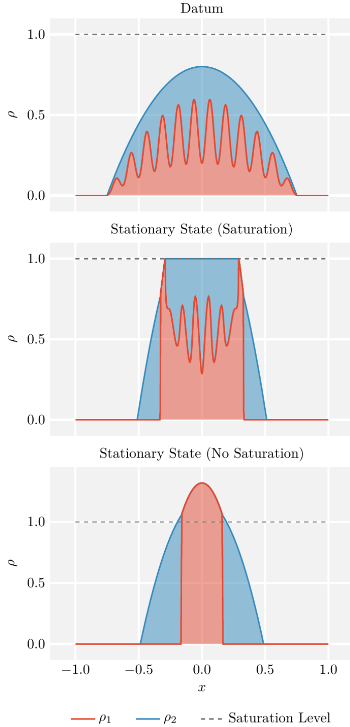
Figure 6: Stationary solutions of Eq. (4.7) in one dimension. \Omega = (-1, 1) , \alpha = 1 , D = 0.1 , C_1 = 4 , C_2 = 2 , \Delta x = 2^{-8} , and \Delta t = 0.1 . Top: datum (4.8). Middle: “frozen-in-place” stationary state with saturation effects. Bottom: segregated stationary state without saturation.
