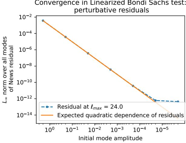
FIG. 6: Residual obtained by subtracting the numerical SpECTRE CCE news from the linearized Bondi-Sachs news. The residual follows closely the expected perturbative residual  $\propto \alpha^2$  for amplitude  $\alpha$ , until the time stepper residual dominates at  $\sim 10^{-12}$  (The absolute tolerance of the time stepper is chosen to be  $10^{-13}$  in these tests and run for a duration of  $5/\nu$ ).
