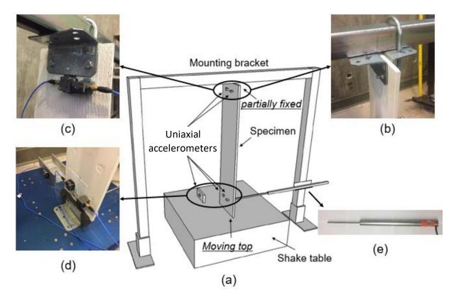
Figure 6: Experiment details: (a) Overall experimental setup; (b) Details of partially fixed support; (c) Details of bottom sensors ( $\theta_2$ ); (d) Details of top sensors ( $\theta_1$ ); and (e) LVDT.
