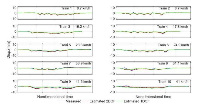
Figure 9. Pseudo-static displacement estimation with 1DOF and 2DOF methods.
