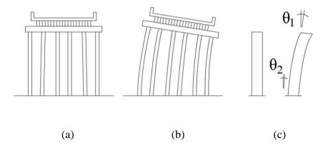
Figure 3. Cantilever simplification for a bridge.
