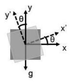
Figure 2. Two axis accelerometer sensing rotation diagram.
