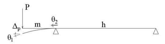
Figure 4. Simplification of the new pile.
