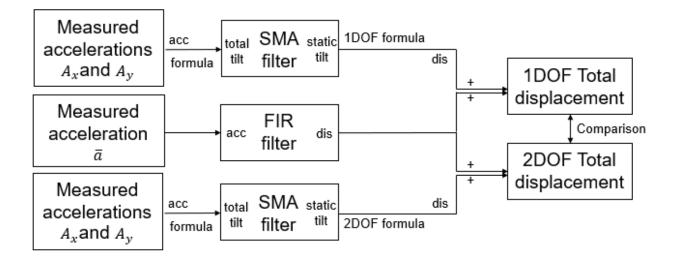
Figure 5. Flowchart comparison between model-free, reference-free 1DOF and 2DOF total displacement estimation.
