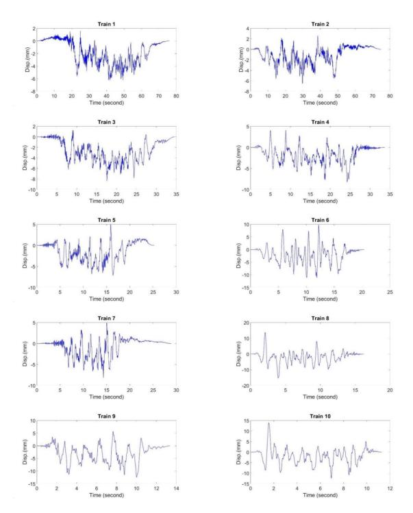
Figure 7. Summary of transverse displacements from ten train-crossing events from the field used for the laboratory experiments.
