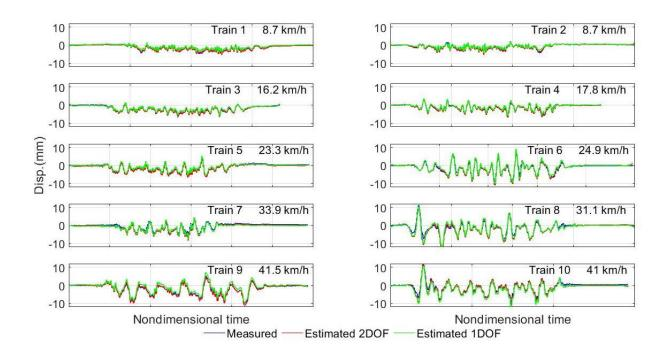
Figure 10. Total displacement estimation with 1DOF and 2DOF methods.
