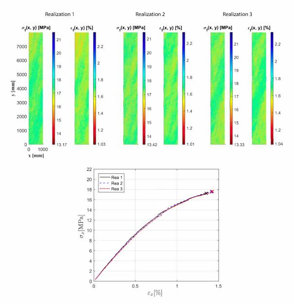
**Figure 19.** Three random realizations of 1 m  $\times$  8 m samples and corresponding uniaxial response.
