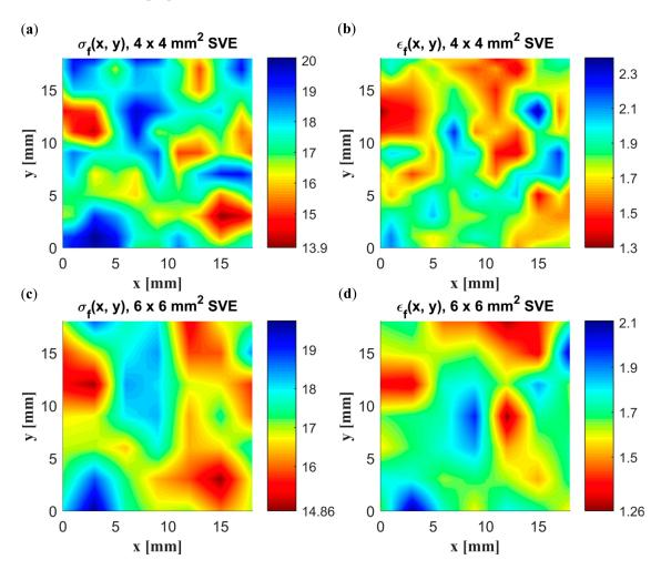
**Figure 13.** Spatial distribution of strength  $\sigma_f$  (MPa) and strain to failure  $\varepsilon_f$  (%) using SVEs of size (a)  $4 \times 4 \text{ mm}^2$  and (b)  $6 \times 6 \text{ mm}^2$  and a discretization distance of half the SVE size.
