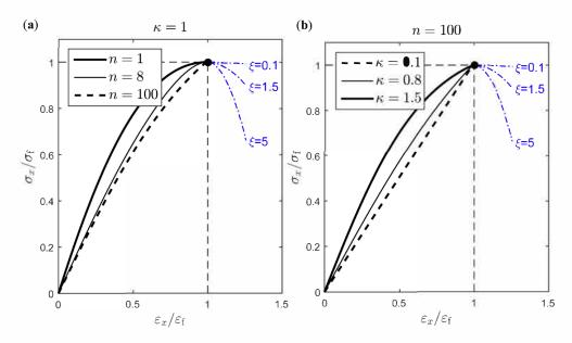
**Figure 6.** Effect on the stress–strain relation of (a) damage exponent n and (b) parameter  $\kappa$  in Equation (23).
