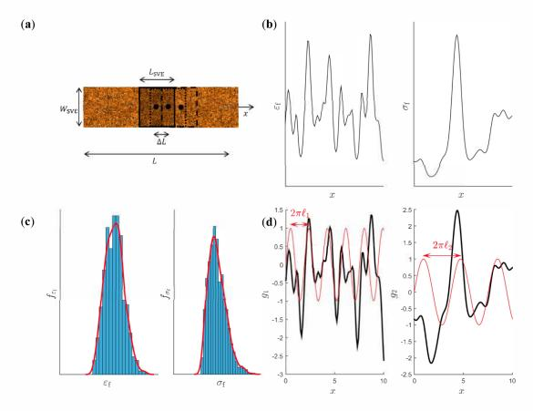
**Figure 5.** (a) Sample used to characterize the spatial random fields of  $\varepsilon_f$  and  $\sigma_f$  with discretization distance  $\Delta L$ . Schematic (b) Spatial random fields of  $\varepsilon_f$  and  $\sigma_f$ . (c) Univariate approximation of the probability density function of  $\varepsilon_f$  and  $\sigma_f$ . (d) Transformed Gaussian random fields.
