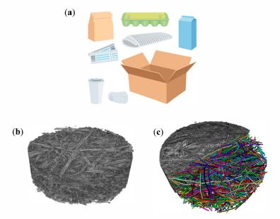
**Figure 1.** (a) Example of fiber-based product, (b) micro-tomography of fiber network, and (c) fiber network schematic reconstruction.
