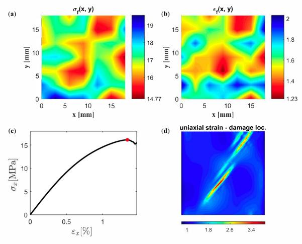
**Figure 16.** Randomly simulated spatial field of (**a**) strength  $\sigma_f(Mpa)$  and (**b**) strain to failure  $\varepsilon_f$  (%); (**c**) uniaxial response; and (**d**) spatial distribution of uniaxial strain at the maximum applied stress (marked by a red point in (**c**)).
