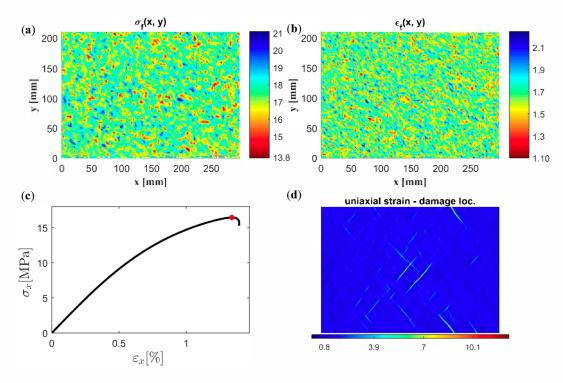
**Figure 17.** Randomly simulated spatial field of (a) strength  $\sigma_f$  (Mpa) and (b) strain to failure  $\varepsilon_f$  (%); (c) uniaxial response; and (d) spatial distribution of uniaxial strain at the maximum applied stress (marked by a red point in (c)).
