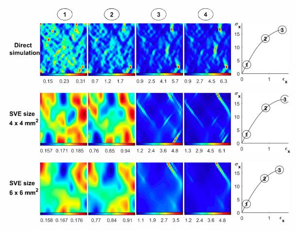
**Figure 15.** Spatial distribution of uniaxial strain with increased loading for: direct simulation, continuum model with SVE size  $4 \times 4$  mm<sup>2</sup>, and continuum model with SVE size  $6 \times 6$  mm<sup>2</sup>.
