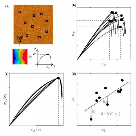
**Figure 7.** (a) SVEs of the same size randomly cut from a thin fiber network. (b) Constitutive response from uniaxial tensile tests on the SVEs. (c) Scaled constitutive response. (d) Parameter  $\kappa$  as a function of  $\varepsilon_f$  and residual error R.
