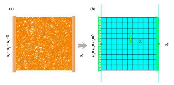
Figure 12. Finite element model and boundary conditions of a uniaxial test using (a) direct fiber simulation and (b) proposed continuum model.
