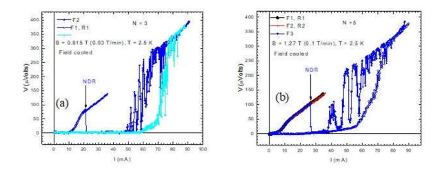
Figure S1: (a) shows onset of NDR after two cycling at 0.815 T (0.03 T/min) at 2.5 K, FC state. (b) shows onset of NDR after 4 cycling at 1.27 T (0.1 T/min) at 2.5 K, FC state.
