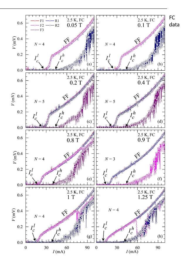
6. Nine *I-V* cyclings. After 4 cycles (F1, R1, F2, R2), the high  $I_c^h$  state is reached (in F3). After that further cycles F3, R3, F4, R4, F5 keeps the system in the high  $I_c^h$  state.
