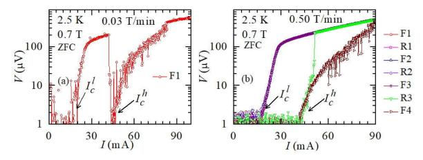
Figure 3. *I-V* data (for F1, R1, F2, R2, F3, R3 and F4 runs) at 2.5 K and 0.7 T (ZFC) for (a)  $\dot{B} = 0.03$  T/min and (b) 0.50 T/min, respectively. The locations of  $I_c^l$  and  $I_c^h$  are marked with arrows. (see text for details)
