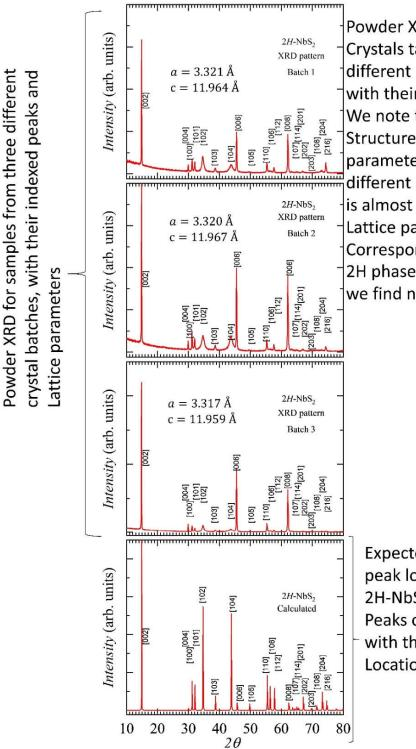
Powder XRD Analysis of Crystals taken from different batches along with their Indexing. We note that the crystalline Structure / lattice parameters, across the different crystal batches is almost uniform. The Lattice parameters Correspond with the 2H phase of NbS2 and we find no 3R phase.
