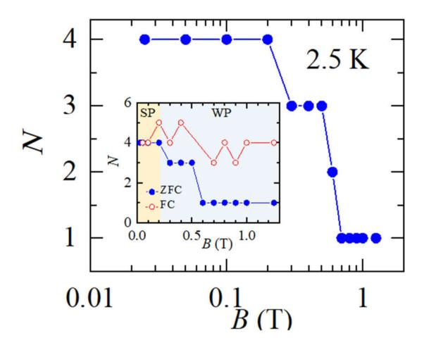
Figure 5. Main panel shows the number of *I* cycles needed for the *I*-*V* to show the NDR transition, i.e., N(B) at 2.5 K (for the static vortex state prepared in the ZFC mode). Inset shows comparison of N(B) values for static vortex state prepared in the FC and ZFC modes at 2.5 K. In the inset, the yellow and blue regions represent the SP and WP regimes (compared with Fig. 1(c)), respectively.
