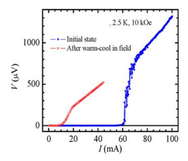
Figure S3: *I-V* response at 2.5 K and 10 kOe of a 2*H*-NbS<sub>2</sub> sample of different batch. The initial state belongs to a zero field cooled vortex state and the after warm-cool state in field corresponds to a field cooled (FC) state
