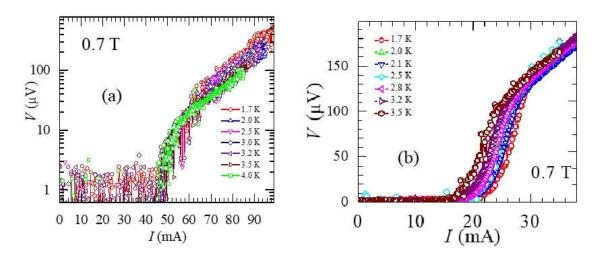
Figure S2: (a) *I-V* data at various *T*'s showing depinning curves across  $I_c^h$ . (b) *I-V* data at various *T*'s showing depinning curves across  $I_c^l$ .
