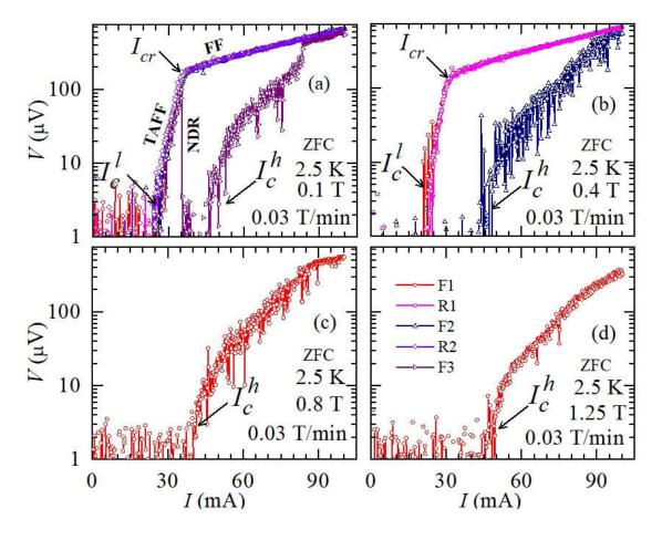
Figure 4. *I-V* data of the driven vortex matter at 2.5 K and (a) 0.01 T, (b) 0.04 T, (c) 0.8 T and (d) 1.25 T. The pristine vortex state is prepared in ZFC mode at B = 0.03 T/min.  $I_c^l$  and  $I_c^h$  locations are marked with arrows. The current cycle legends shown in (d) are retained the same for (a)-(d).
