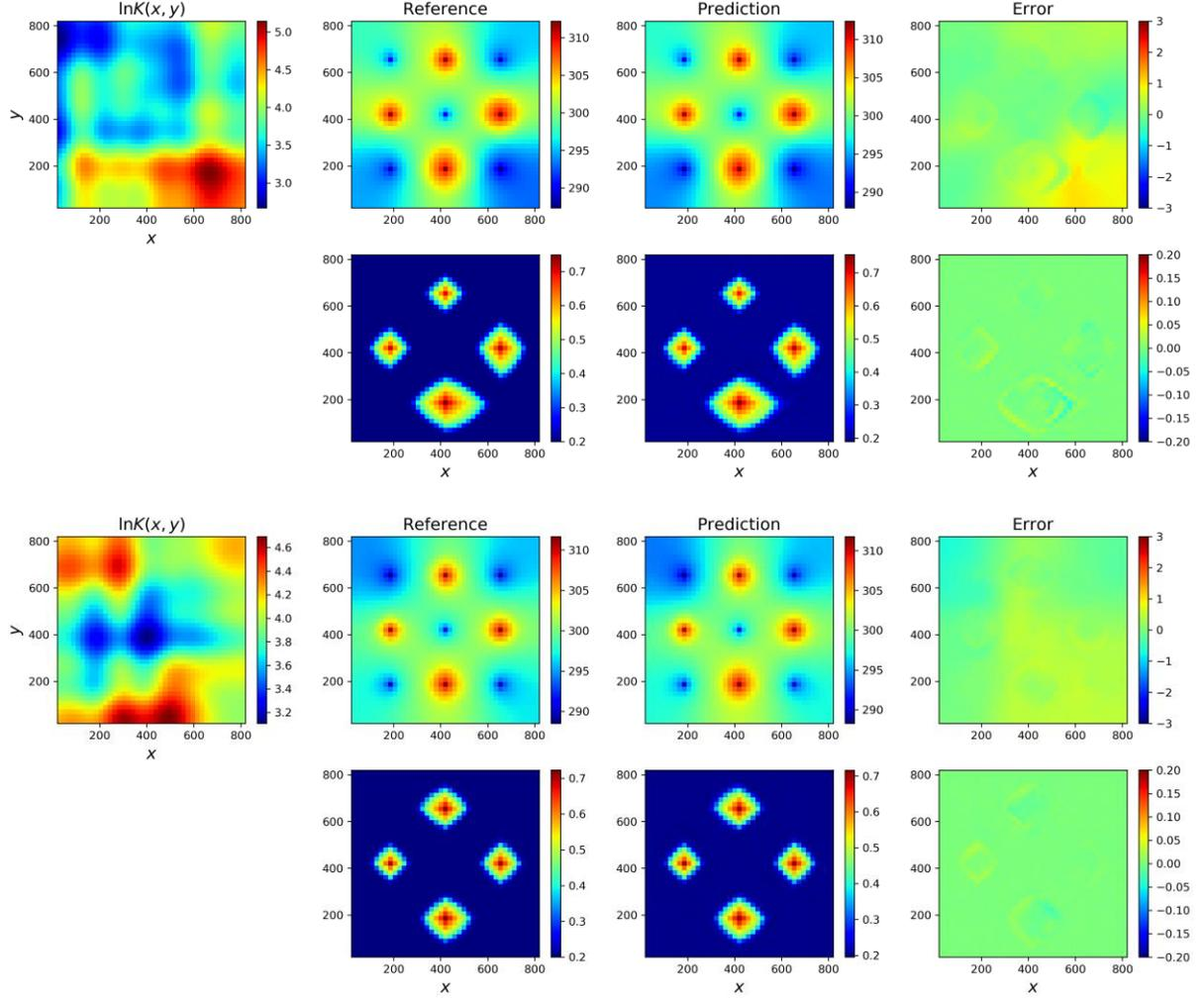
**Figure 4.** Predictions and references of pressure and saturation distribution for three different permeability fields.
