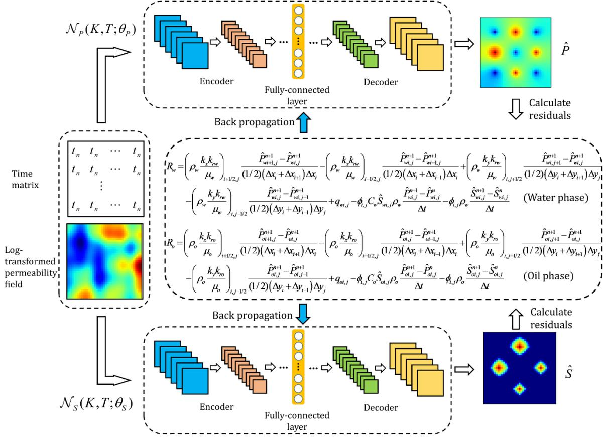
Figure 1. Framework of TgCNN for two-phase flow.
