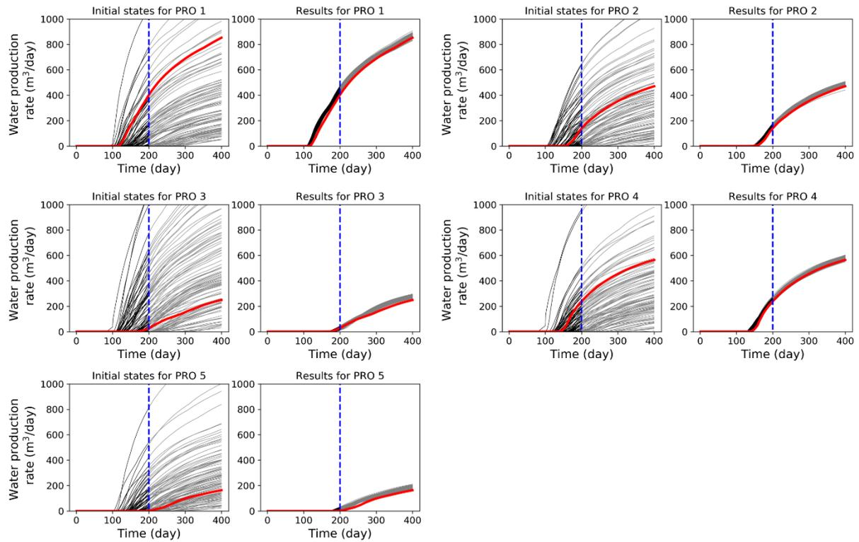
**Figure 18.** Water production data matching and prediction results. The red lines denote the water production rate for the reference realization. The blue dashed lines separate the data matching phase and the prediction phase. The black lines before the blue dashed lines denote the production rate of different realizations in the data matching phase, and the gray lines after the blue dashed lines denote the production rate of different realizations in the prediction phase.
