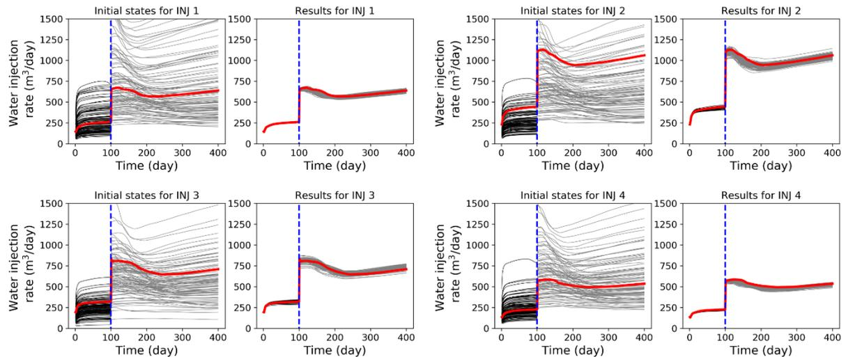
**Figure 16.** Water injection data matching and prediction results. The red lines denote the water injection rate for the reference realization. The blue dashed lines separate the data matching phase and the prediction phase. The black lines before the blue dashed lines denote the water injection rate of different realizations in the data matching phase, and the gray lines after the blue dashed lines denote the water injection rate of different realizations in the prediction phase.
