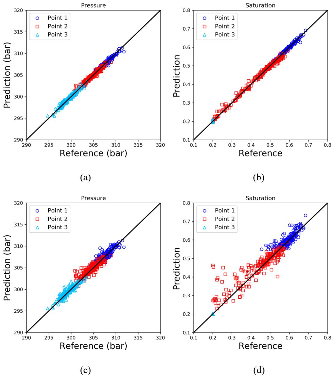
**Figure 5.** Scatter plots of reference values and predictions from TgCNN and CNN surrogates: (a) pressure with TgCNN; (b) saturation with TgCNN; (c) pressure with CNN; (d) saturation with CNN.
