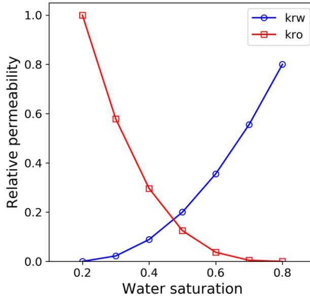
**Figure 3.** Relative permeability curves of the oil and water phase.
