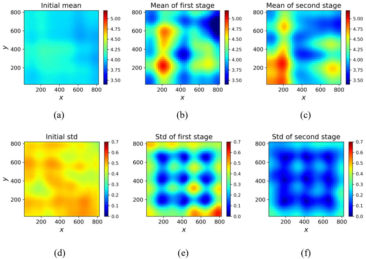
**Figure 13.** (a) Mean of initial realizations; (b) mean of estimated permeability fields with production data of the first 100 days; (c) mean of estimated permeability fields with production data of 200 days; (d) standard deviation of initial realizations; (e) standard deviation of estimated permeability fields with production data of the first 100 days; (f) standard deviation of estimated permeability fields with production data of 200 days.
