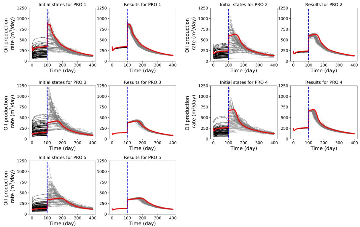
**Figure 14.** Oil production data matching and prediction results. The red lines denote the oil production rate for the reference realization. The blue dashed lines separate the data matching phase and the prediction phase.
