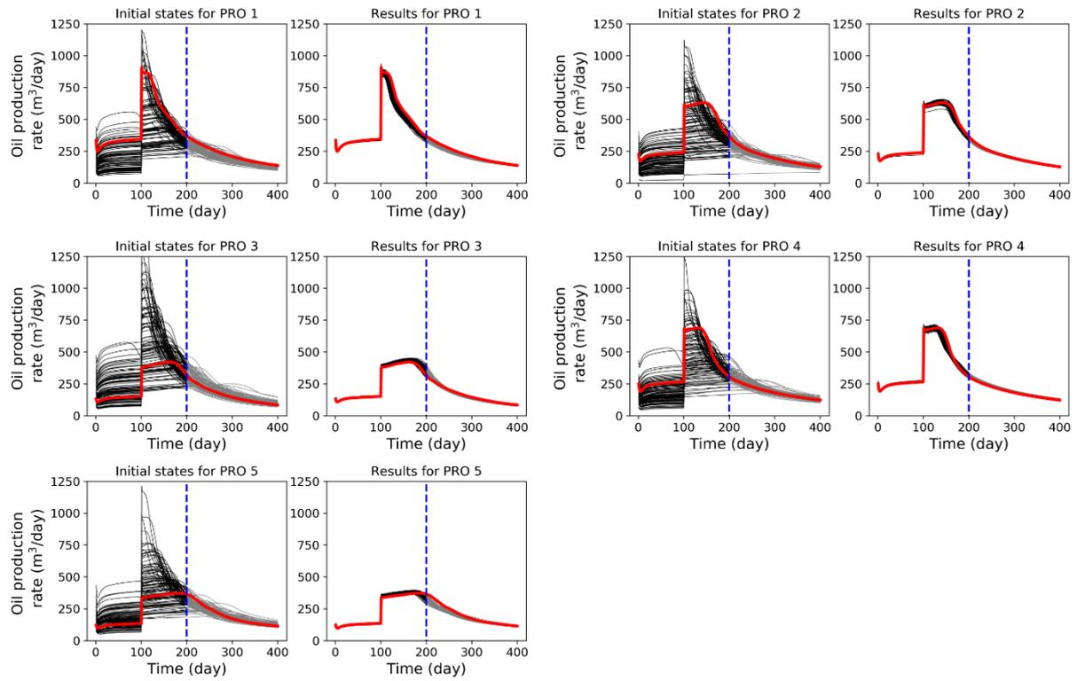
**Figure 17.** Oil production data matching and prediction results. The red lines denote the oil production rate for the reference realization. The blue dashed lines separate the data matching phase and the prediction phase.
