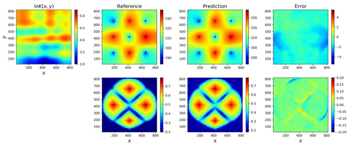
**Figure 8.** Predictions and references of pressure and saturation distribution for the sampled permeability field.
