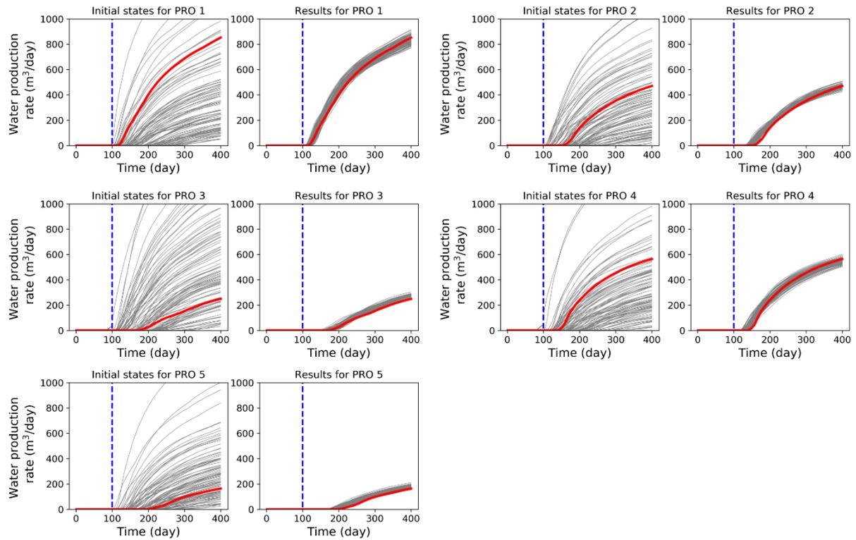
**Figure 15.** Water production data matching and prediction results. The red lines denote the water production rate for the reference realization. The blue dashed lines separate the data matching phase and the prediction phase. The black lines before the blue dashed lines denote the production rate of different realizations in the data matching phase, and the gray lines after the blue dashed lines denote the production rate of different realizations in the prediction phase.
