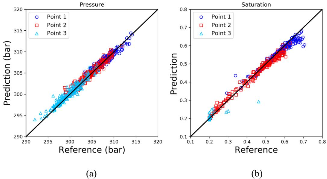
**Figure 11.** Scatter plots of reference values and predictions from TgCNN for (a) pressure and (b) saturation.
