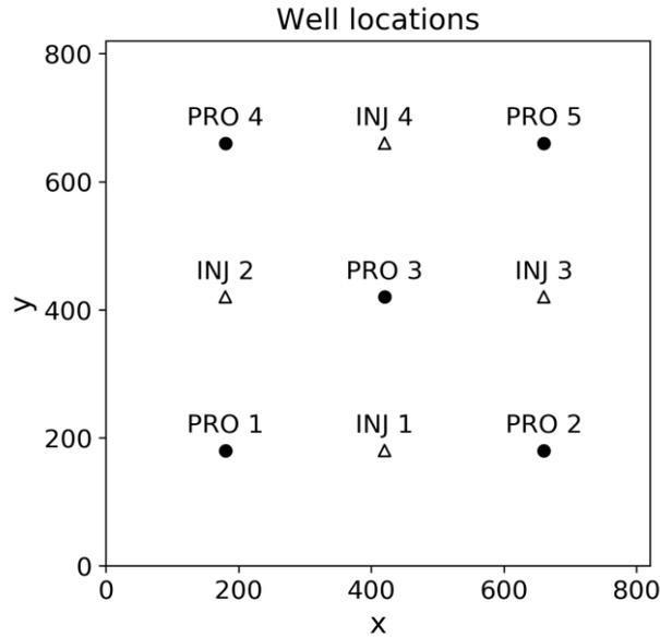
**Figure 2.** Well locations of the water-flooding problem. The filled circles denote the producers and the empty triangles denote the injectors.
