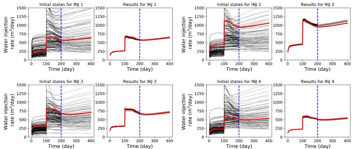
**Figure 19.** Water injection data matching and prediction results. The red lines denote the water injection rate for the reference realization. The blue dashed lines separate the data matching phase and the prediction phase. The black lines before the blue dashed lines denote the water injection rate of different realizations in the data matching phase, and the gray lines after the blue dashed lines denote the water injection rate of different realizations in the prediction phase.
