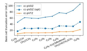
FIG. 2. Basis set truncation errors for the cc-pVDZ and cc-pVTZ basis sets for a range of hydrocarbons, compared with the truncation error for a reoptimized cc-pVDZ basis set. The reference energies are computed in the cc-pV5Z basis set. None of the molecules shown in the figure were used in the basis set optimization.
