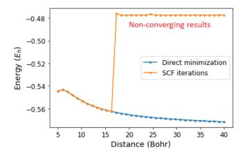
FIG. 1. Unrestricted PW92/cc-pVDZ [27, 28] energy for the hydrogen molecule cation  $H_2^+$  as a function of the internuclear distance calculated via the SCF (using Broyden's method [24]) and direct minimization approaches. Note that the SCF iterations do not converge for internuclear distances larger than 17 Bohr.
