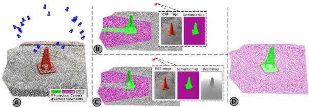
Figure 2. Proposed semantic digital twining to detect objects of interest.
