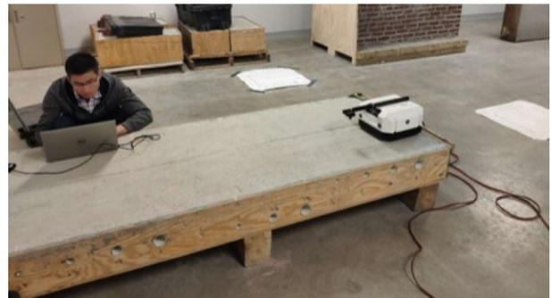
Figure 1. Picture of our inspector and the robot inspecting a slab at a test field.
