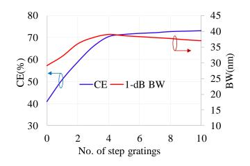
Fig. 3. Coupling efficiency at wavelength of 1550 nm and bandwidth for number of steps gratings into the primary grooves.
