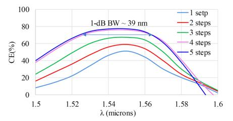
Fig. 11. Coupling efficiency vs. wavelength for optimized grating coupler with various numbers of step gratings in the primary groove.
