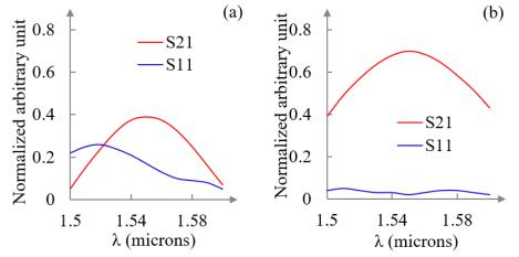
Fig. 7. Reflection (S11) and transmission (S21) with different wavelengths for vertical incident in (a) GC with only primary grating (b) GC with engineered sub-wavelength grating. Vertical axis is normalized to incident field intensity.
