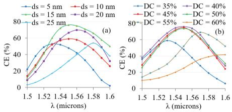
Fig. 9. Coupling efficiency vs wavelength for various (a) secondary etch depth ( $d_s$ ) and (b) secondary duty cycle ( $DC_s$ ).
