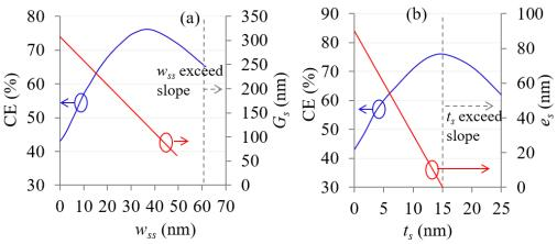
Fig. 10. Coupling efficiency for various (a) widths and corresponding groove spaces (b) thicknesses and corresponding etch spaces at 1550 nm wavelength.
