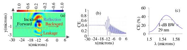
Fig. 5. (a) E-field distribution along grating structure (b) coupling efficiency at wavelength of 1550 nm and (c) coupling bandwidth.
