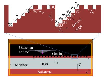
Fig. 2. 2D FDTD simulation environment setup. Inset: geometry of the secondary gratings (drawing not to scale).
