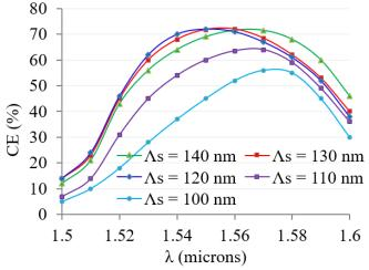
Fig. 8. Coupling efficiency vs wavelength for various secondary grating period.
