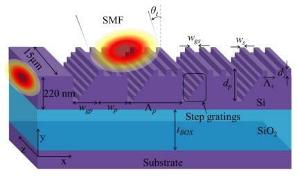
Fig. 1. Geometry of the proposed engineered subwavelength grating coupler (drawing not to scale).
