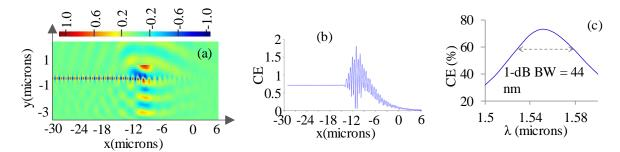
Fig. 6. (a) E-field distribution along grating structure (b) coupling efficiency at wavelength of 1550 nm and (c) coupling bandwidth for grating coupler with secondary ultra-subwavelength grating.
