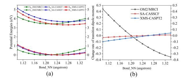
**Figure S4**. Potential energy curves (a) and the change of  $S_0 \rightarrow S_1$  transition dipole moments (b) as functions of the NN distance. The change of the transition dipole moment at the optimized geometry is set to zero.
