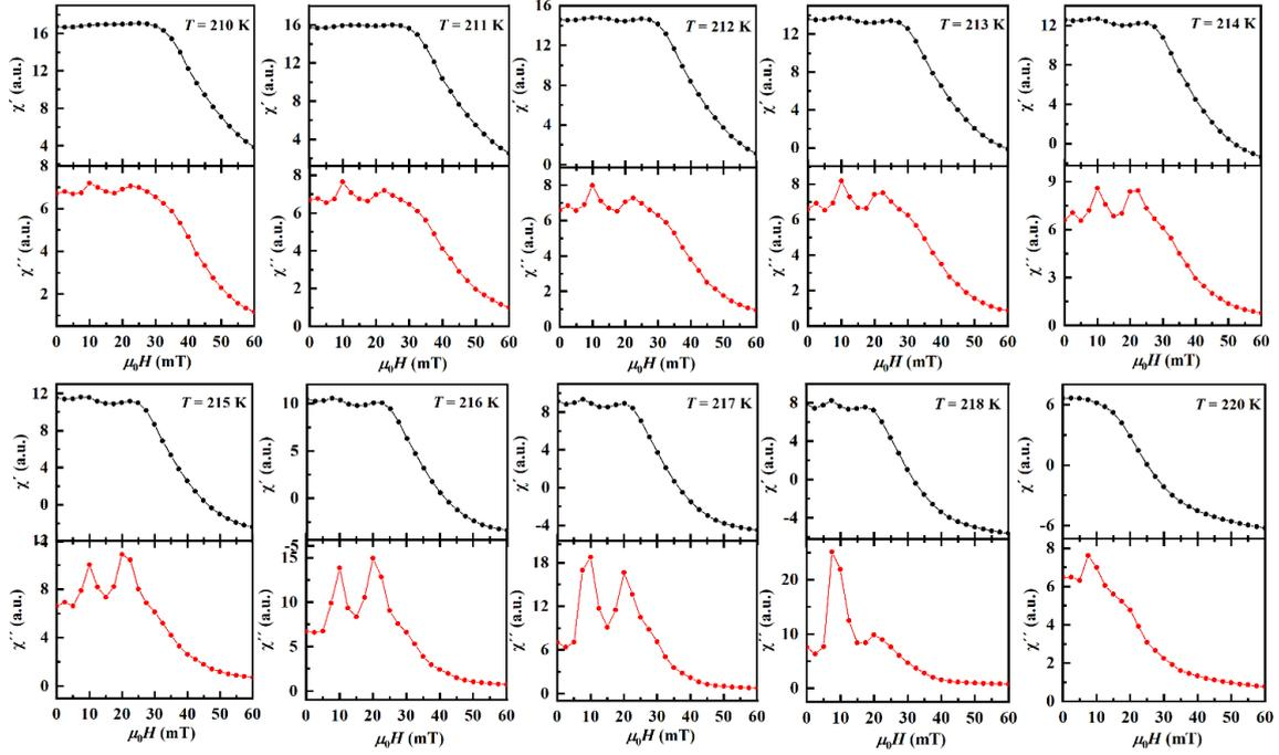
**FIG. S3** Magnetic-field dependence of  $\chi'$  and  $\chi''$  of  $\text{Co}_7\text{Zn}_8\text{Mn}_5$  alloy for some selected temperatures after zero-field cooling.
