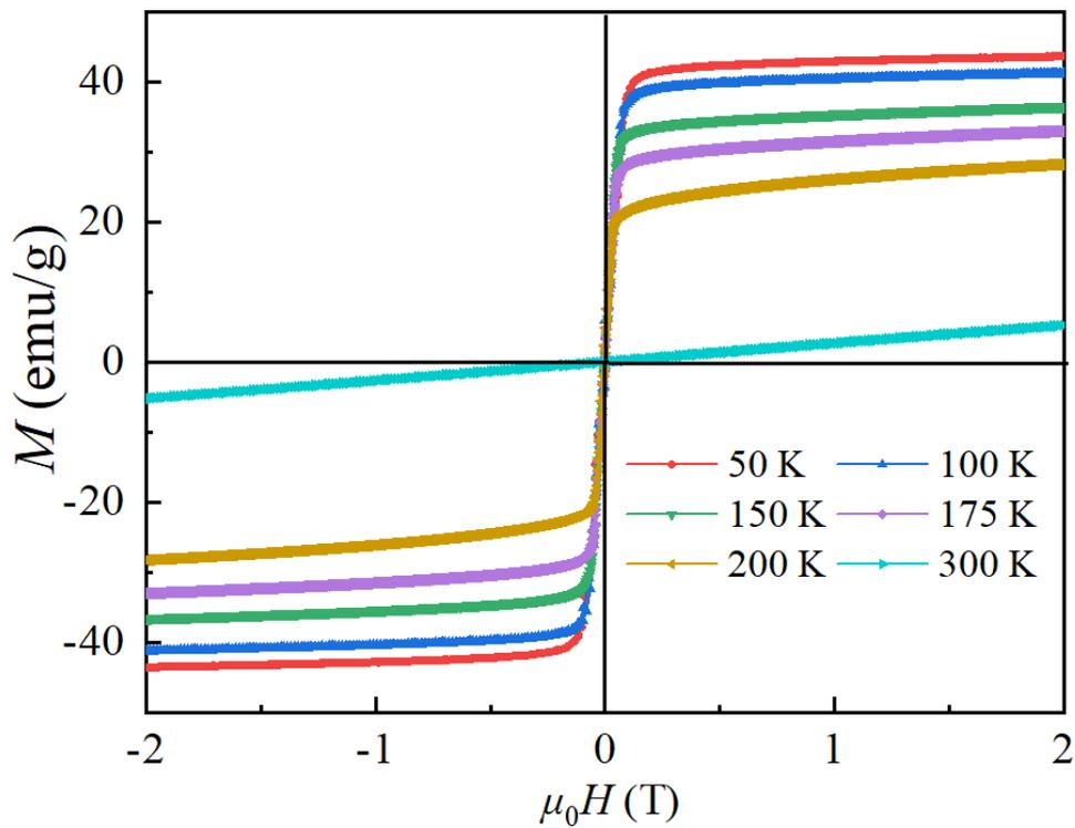
**FIG. S2** Isothermal hysteresis loop curves at different temperatures.
