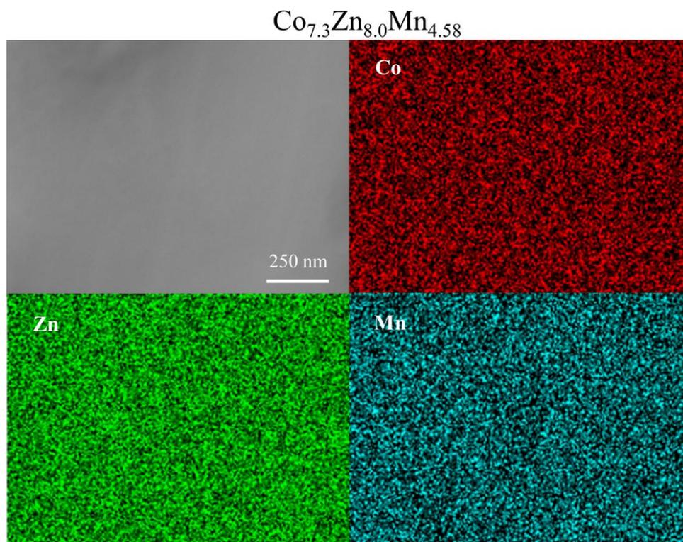
**FIG. S1** Two-dimensional mappings of constituent elements, Co, Zn, and Mn, in terms of Energy dispersive X-ray spectroscopy (EDX) for  $\text{Co}_7\text{Zn}_8\text{Mn}_5$  alloy.
