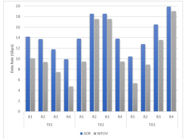
Figure 4 Achievable data rate when using ADR and WFOV receivers
