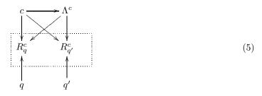
An arrow here indicates that the distribution of its terminal node may change with the value of its initial node, and the dotted box indicates that the random variables within it are jointly distributed.
