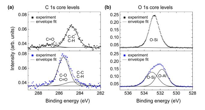
**Figure S3.** (a) Carbon 1s (C 1s) and (b) oxygen 1s (O 1s) core level spectra of solvent-cleaned bare *p*-doped Si (top, black squares) and *p*-Si substrates after exposure to 20 cycles (bottom, blue squares).
