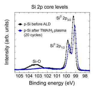
**Figure S4.** Silicon 2p core level spectra of silicon substrates without (black) and with (blue) an alumina layer deposited by ALD following 20 cycles of TMA and remote H<sub>2</sub> plasma. The intensity of detected photoelectrons is not normalized in this plot.
