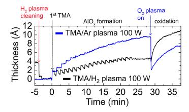
**Figure S1.** Thickness of surface oxide layers as a function of time plot obtained from *in-situ* SE on Si substrates with a native SiO<sub>2</sub> layer during 20 cycles of the TMA/H<sub>2</sub> (black line) and TMA/Ar plasma (blue line) process at 200 °C and 100 W plasma power. The oxygen plasma treatment was carried out at 100 W plasma power and a 20 sscm flow rate and 0.04 Torr background pressure.
