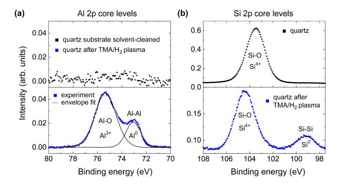
**Figure S5.** X-ray photoelectron spectra of the (a) Al 2p and (b) Si 2p core levels of a representative solvent-cleaned quartz substrate (top row, black squares) and quartz substrates after TMA/H<sub>2</sub>
