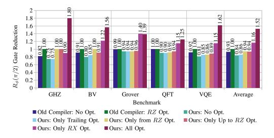
Fig. 3. Comparison of reduction in  $R_{\phi}(\pi/2)$  operations generated across our benchmarks by the existing compiler and by other compiler configurations (higher is better). We calculate reduction by dividing the  $R_{\phi}(\pi/2)$  gates the existing compiler generates with RZ optimizations enabled by the number of  $R_{\phi}(\pi/2)$  gates generated by some other configuration. We include the existing compiler without optimizations for comparison.
