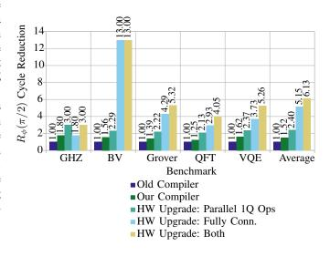
Fig. 6. Comparison of reduction in  $R_{\phi}(\pi/2)$  operations generated across our benchmarks by our compiler between present hardware and different hardware upgrades (higher is better).
