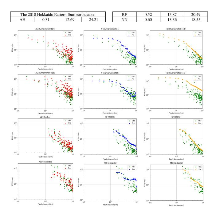
Fig. 5. Observations (Obs) and predictions (Pre) of the 4 recent earthquakes by predictors of the the attenuation equation (AE), random forest (RF), neural network (NN). Red points represent the prediction by the attenuation equation; blue points represent the prediction by the random forest predictor; orange points represent the prediction by the neural network predictor; and green points represent the observed data, respectively.
