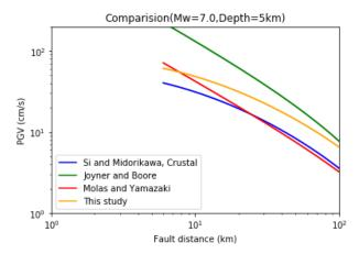
Fig. 2. Comparison of attenuation equations for PGV of this study and previous studies for magnitude 7.0 earthquake with the depth of 5 km.
