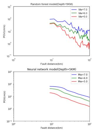
Fig. 3. Predicted attenuation curves for PGV obtained by the regression analysis, random forest, and neural network for the magnitudes of 5.0, 6.0 and 7.0 earthquakes with depth of 5 km.
