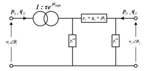
Fig.1 The standard  $\pi$  model for a branch.
