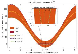
Fig.4 Branch reactive power on AS<sup>Q</sup> and RS<sup>Q</sup> (Reactive Power).
