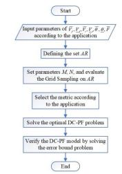
Fig.7 The flowchart of optimal DC-PF method.
