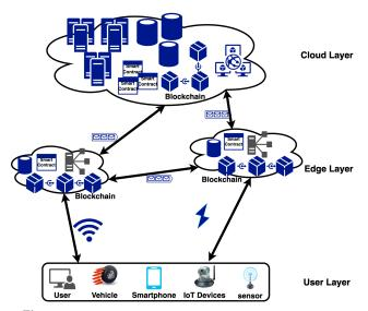
**Figure 1:** General blockchain based edge computing framework. contract's operating status and financial costs. In addition to combining game theory and Nash equilibrium theory[33], the system can make optimal decisions with minimum costs.
